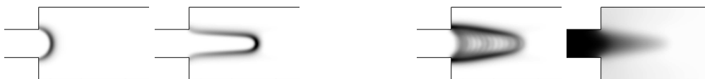
FIGURE 2. Heat release when the flame is the shortest (most left) and the longest (second on the left) during the cycle of oscillation. The above illustrates time averaged heat release (first on the right) and temperature (most right).
