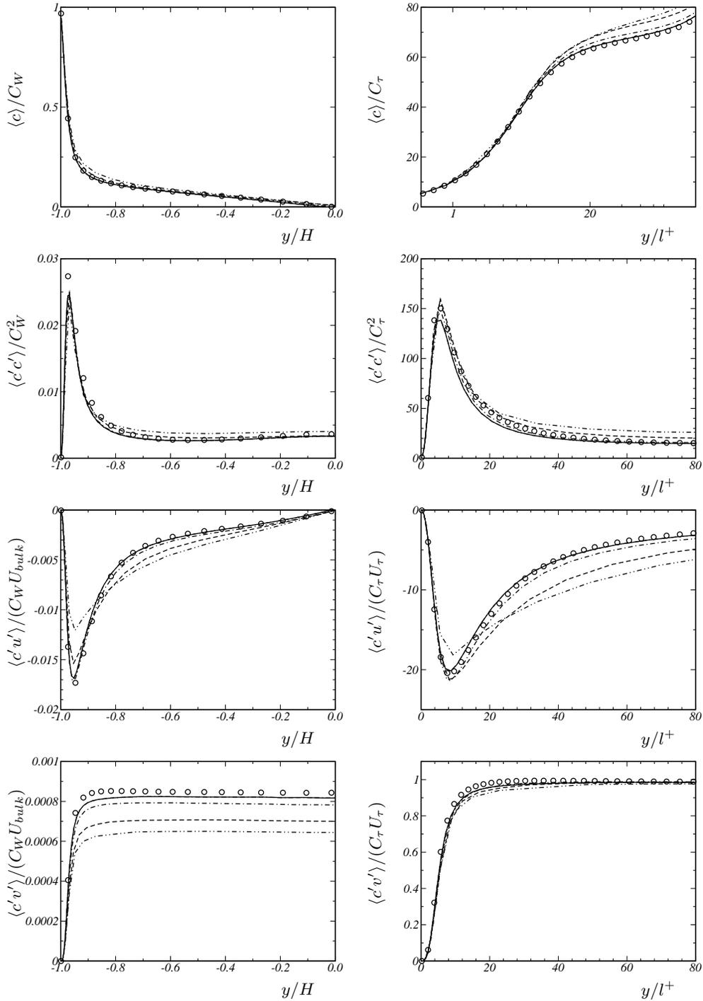
FIGURE 10. Grid-convergence study for implicit LES of passive-scalar transport in turbulent channel flow at  $Re_\tau = 180$  and  $Sc = 10$ . Implicit LES using the high Schmidt number SALD method on a grid with —  $64^3$  cells, ····  $48^3$  cells, - - -  $32^3$  cells, ····  $24^3$  cells.  $\circ$  DNS of Schwertfirm and Manhart (2006)
