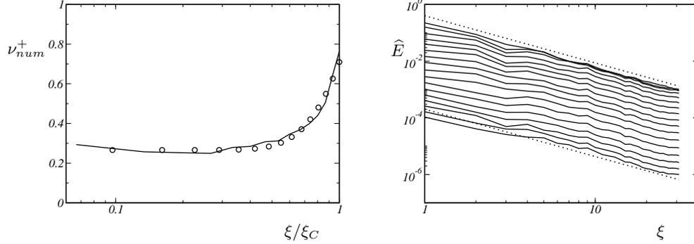
FIGURE 3. Implicit LES of decaying homogeneous isotropic turbulence at the inviscid limit. *Left:* Numerical viscosity of ALDM with optimized parameters compared to the prediction of turbulence theory. — implicit LES with ALDM ;  $\circ$  EDQNM theory (Chollet 1984). *Right:* Instantaneous 3-D energy spectra. — ALDM ; .....  $\hat{E} \sim \xi^{-5/3}$ .
