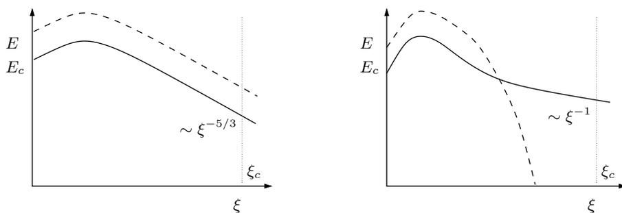
FIGURE 1. Critical test cases for predicting the proper subgrid diffusion in large-eddy simulations of scalar mixing. *Left*: Low Schmidt number regime. *Right*: High Schmidt number regime at moderate Reynolds number. — scalar variance ; - - - kinetic energy.
