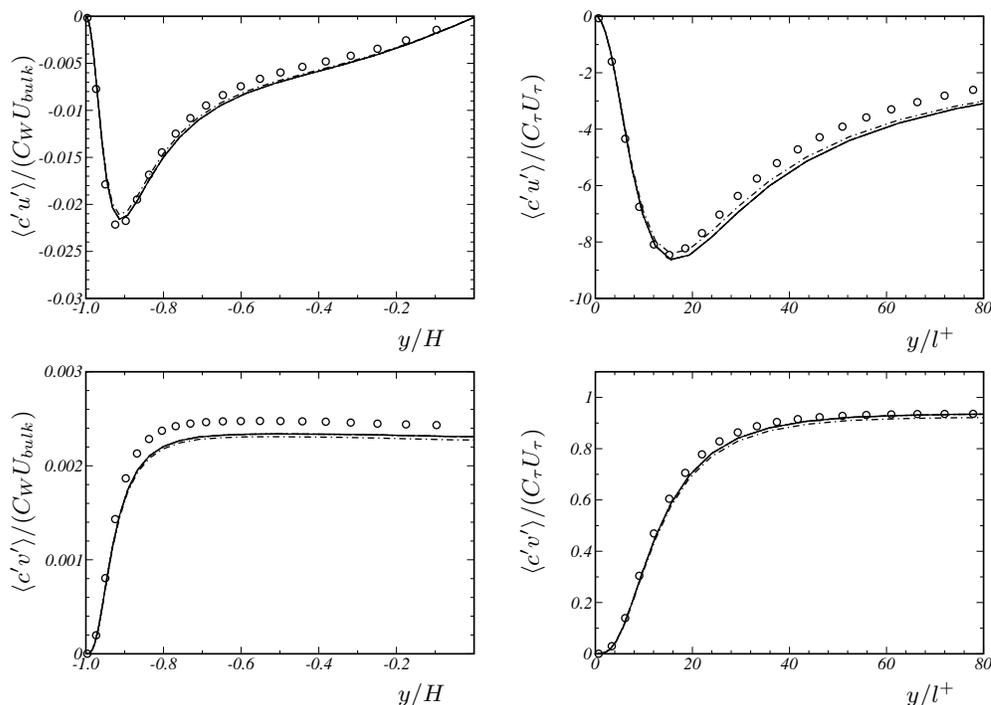
FIGURE 8. Turbulent transport of a passive scalar in plane channel flow at  $Re_\tau = 180$  and  $Sc = 1$ . Implicit LES with parameters optimized for — high Schmidt numbers, - - - low Schmidt numbers,  $\circ$  DNS of Schwertfirm and Manhart (2006).
