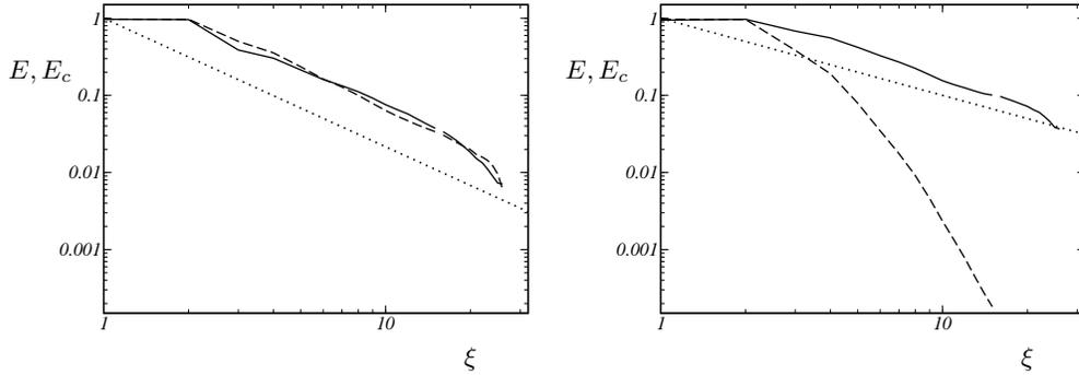
FIGURE 4. Mean 3-D spectra of kinetic energy and scalar variance for implicit LES of large-scale forced isotropic turbulence. *Left*:  $Re = 10^4$  and  $Sc = 1$ . *Right*:  $Re = 20$  and  $Sc = 400$ . — scalar variance; - - - kinetic energy; ..... analytical expressions for scalar variance.
