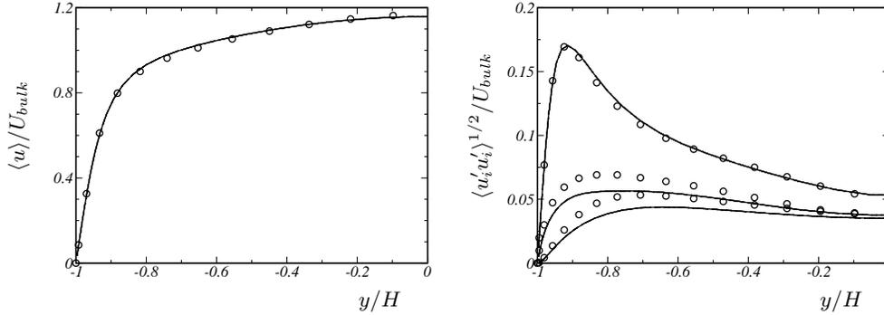
FIGURE 5. Mean velocity profile and Reynolds stresses in turbulent channel flow at  $Re_\tau = 180$ . — implicit LES with SALD,  $\circ$  DNS data of Moser *et al.* (1999).
