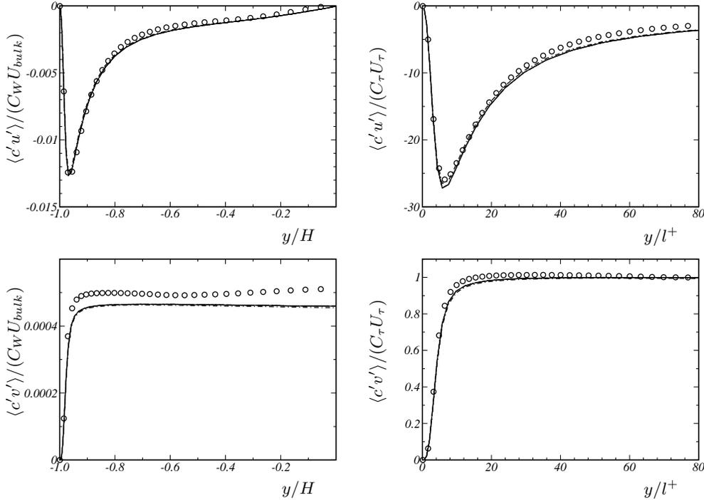
FIGURE 9. Turbulent transport of a passive scalar in plane channel flow at  $Re_\tau = 180$  and  $Sc = 25$ . Implicit LES with parameters optimized for — high Schmidt numbers, - - - low Schmidt numbers,  $\circ$  DNS of Schwertfirm and Manhart (2006).
