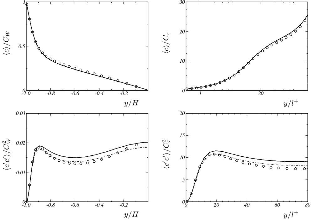
FIGURE 6. Profiles of mean scalar concentration and scalar variance in plane channel flow at  $\text{Re}_\tau = 180$  and  $\text{Sc} = 1$ . Implicit LES with parameters optimized for — high Schmidt numbers, - - - low Schmidt numbers,  $\circ$  DNS of Schwefirm and Manhart (2006).
