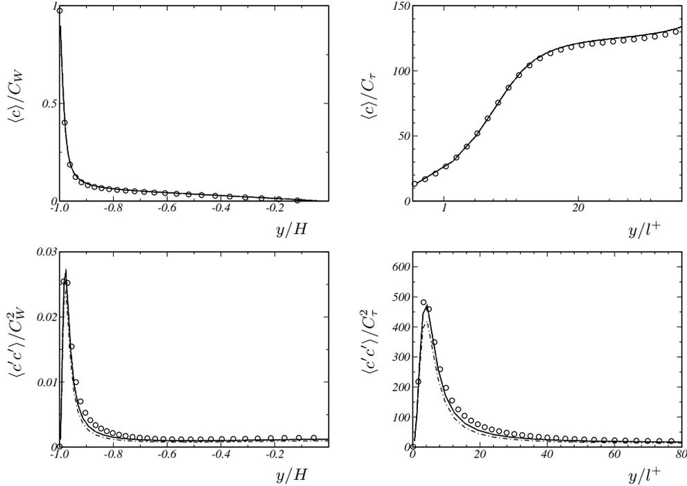
FIGURE 7. Profiles of mean scalar concentration and scalar variance in plane channel flow at  $Re_\tau = 180$  and  $Sc = 25$ . Implicit LES with parameters optimized for ——— high Schmidt numbers, - · - · - low Schmidt numbers,  $\circ$  DNS of Schwefirm and Manhart (2006).
