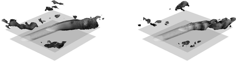
FIGURE 6. Instantaneous iso-surface of velocity modulus ( 1.125 V_j ) colored by the normal velocity component (scale is from -0.18 V_j (white) to 0.71 V_j (black)) for the AVBP-1H run at two different instants.
