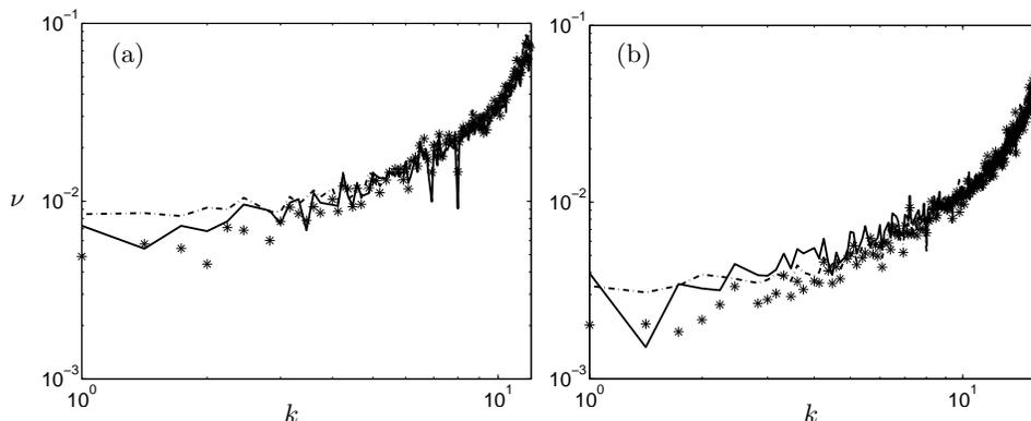
FIGURE 8. Model predictions of the eddy viscosity using the first set of DNS data and synthesized data for the model. Legend: — DNS; \*, current model with randomized DNS data; - · -, current model with synthesized data from Kolmogorov spectrum. (a)  $k_0 = 12$ , (b)  $k_0 = 16$ .
