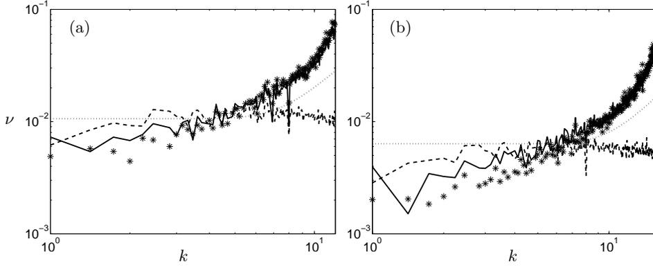
FIGURE 6. Model predictions of the eddy viscosity using the first set of DNS data. Legend: — DNS; --, Smagorinsky model, ···, EDQNM; \* our model (a)  $k_0 = 12$ , (b)  $k_0 = 16$ .
