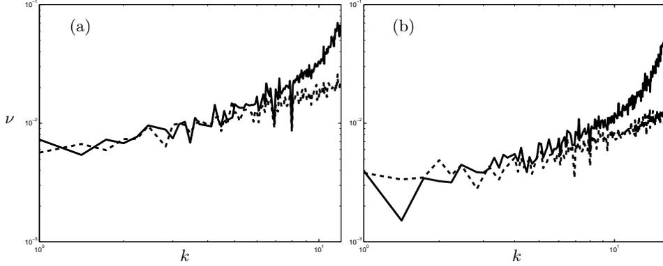
FIGURE 2. Multi-scale method (Novikov and Bodony 2005) performance for two different cutoff wavenumbers. (a)  $k_0 = 12$ , (b)  $k_0 = 16$ . Legend: —,  $\nu_{\text{dns}}$ ; --,  $\nu$  computed using the multi-scale algorithm.
