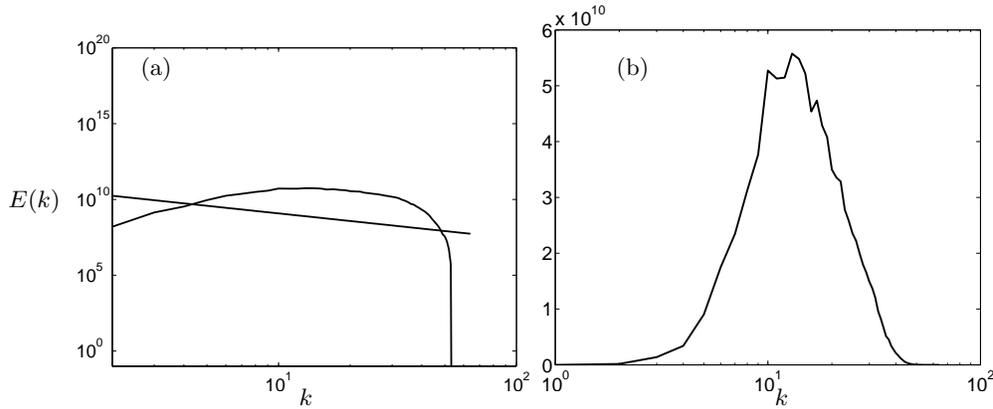
FIGURE 5. Energy spectrum of second set of DNS data (a) log-log scale, (b) log-linear scale.
