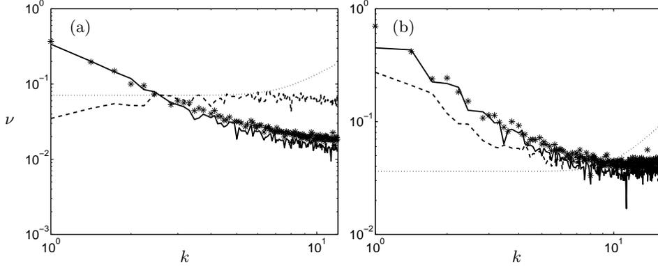
FIGURE 7. Model predictions of eddy viscosity using second set of DNS data. Legend: —, DNS; --, Smagorinsky model; ···, EDQNM; \* current model. (a)  $k_0 = 12$ , (b)  $k_0 = 16$ .
