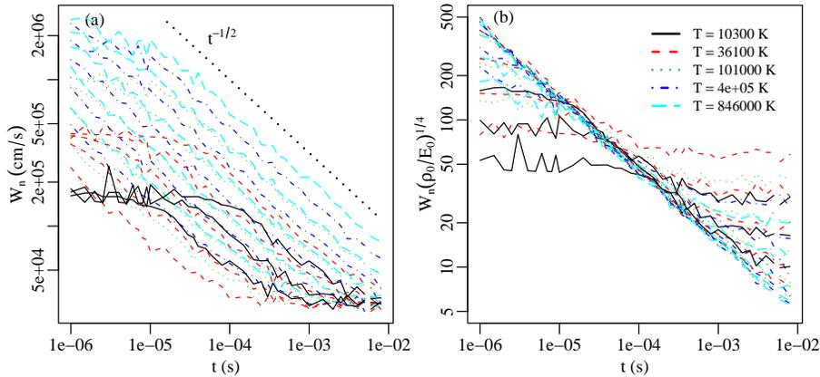
FIGURE 2. Evolution of the shock velocity  $W_n$ ; (a) in cm/s, (b) normalized by  $(E_0/\rho_0)^{1/4}$ .
