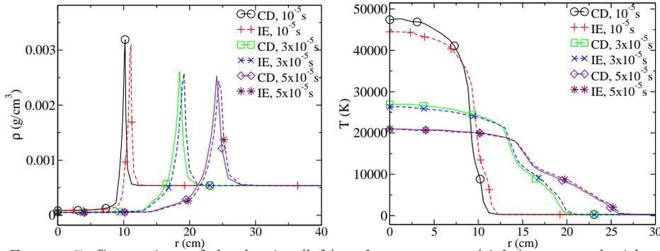
FIGURE 7. Comparison of the density (left) and temperature (right) computed with an initial energy input (EI) vs. using the capacitor discharge model (CD). 17 kJ/cm has been released.
