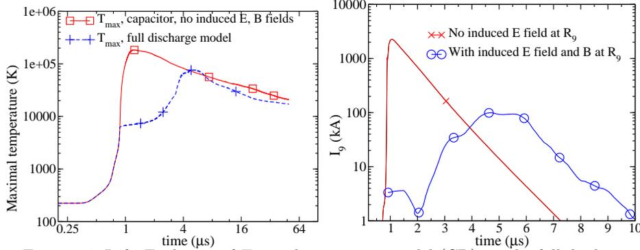
FIGURE 4. Left: Evolution of  $T_{max}$ ; the capacitor model (CD) vs. the full discharge model (FM). Right: Evolution of the current (radius  $R_0$ ) computed with the CD and FM models.
