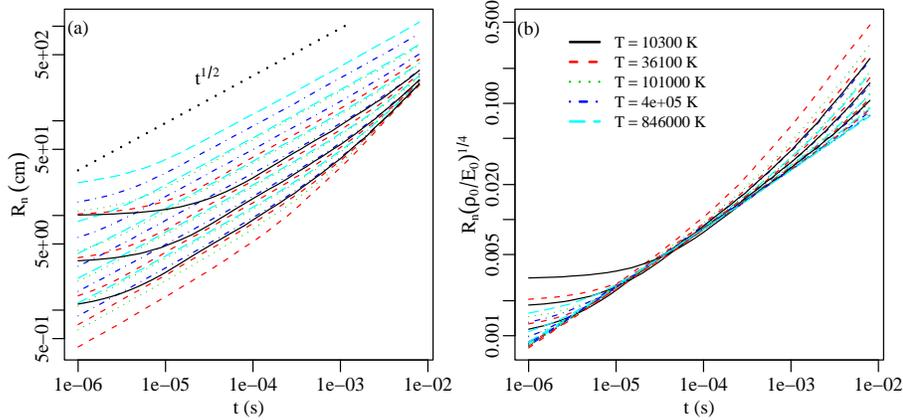
FIGURE 1. Evolution of the shock position  $R_n$ ; (a) in cm, (b) normalized by  $(E_0/\rho_0)^{1/4}$ .
