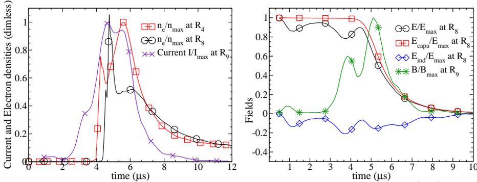
FIGURE 5. Evolution of the dimensionless electron density and current (left) and of the dimensionless electric and magnetic fields (right), computed with the full discharge model.
