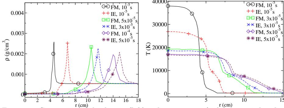
FIGURE 8. Comparison of the density (left) and temperature (right) computed with an initial energy input (EI) vs. using the full lightning discharge model (FM). 2.5 kJ/cm has been released.
