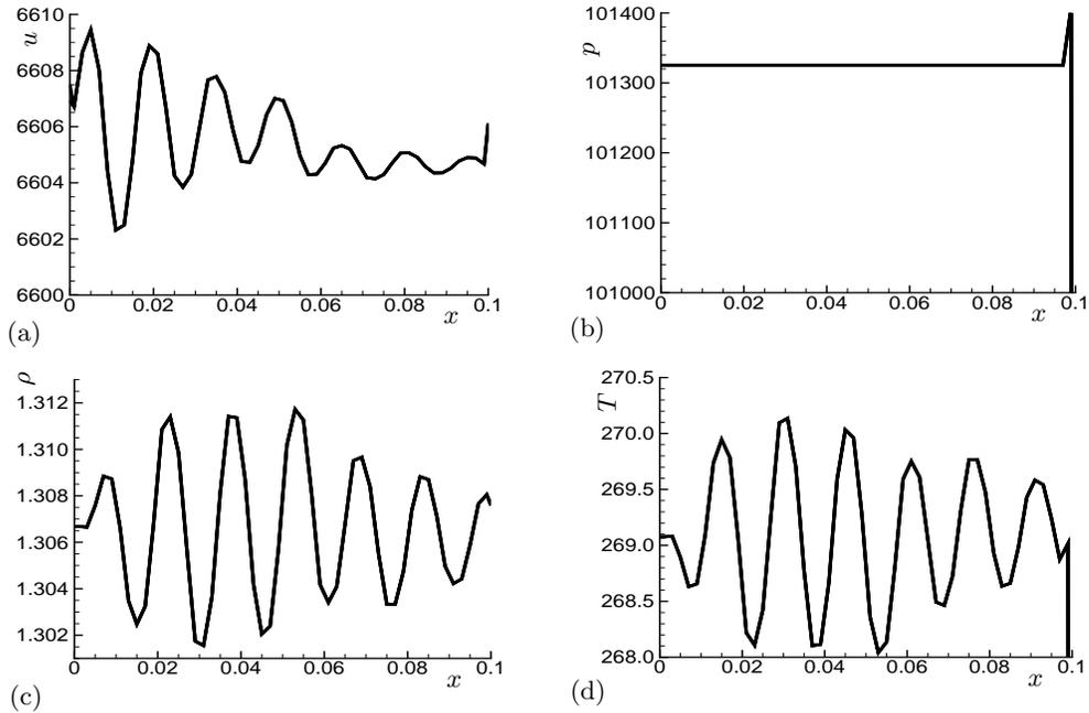
FIGURE 6. Case III: disturbance evolution for a entropic disturbance before the shock. (a) velocity  $u$ , (b) pressure, (c) density  $\rho$ , (d) temperature  $T$ .
