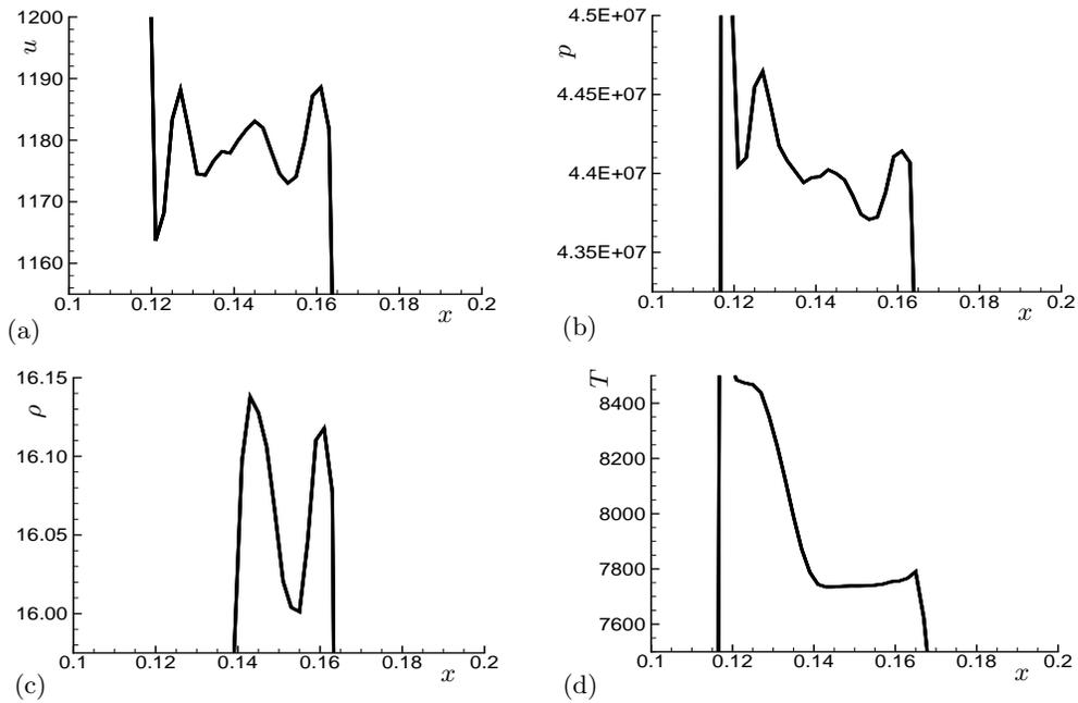
FIGURE 7. Case III: disturbance evolution for a entropic disturbance after the shock. (a) velocity  $u$ , (b) pressure, (c) density  $\rho$ , (d) temperature  $T$ .
