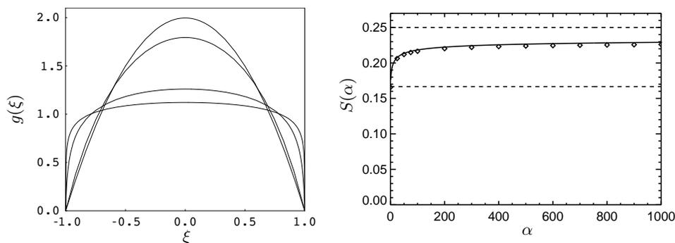
FIGURE 2. Sensitivity of the longitudinal flux flow meter: (Left) model profiles given by Eq. (2.14) and (right) sensitivity  $S(\alpha)$  according to Eq. (2.15). The model profiles are plotted for  $\alpha = 10^{-2}, 10^0, 10^2, 10^4$  (from top to bottom). The diamonds (right) represent the sensitivity computed numerically with the CDP code (see Section 2.2 for details).
