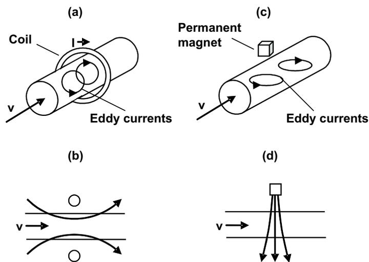
FIGURE 1. Sketch of the two problems considered: Longitudinal flux flowmeter (a), (b) and transverse flux flowmeter (c), (d). The shape of the primary magnetic field is shown in (b) and (d).
