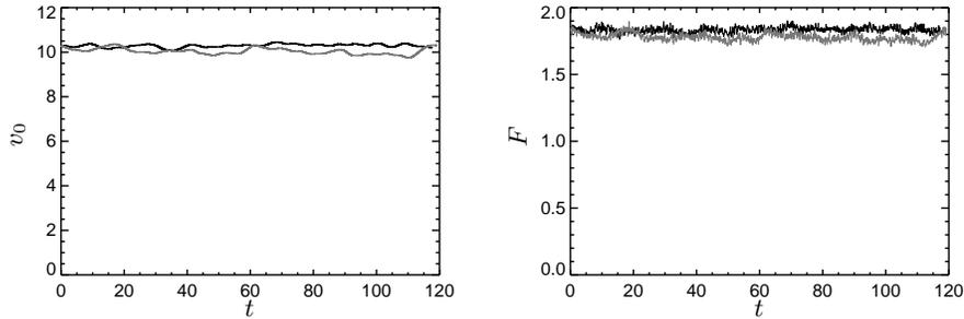
FIGURE 3. Time histories of (a) average velocity  $v_0$  and (b) integrated Lorentz force  $F$  for the unsteady turbulent pipe and longitudinal flux flowmeter. Both plots contain the kinematic (dark line) and MHD (gray line) cases.
