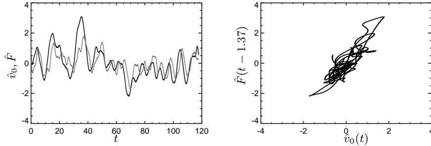
FIGURE 6. Left: time history of the low-pass filtered signals  $\hat{v}_0$  (grey line) and  $\hat{F}$  (dark line). Only the kinematic simulation is considered. Right:  $\hat{F}(t - 1.37)$  as a function of  $\hat{v}_0(t)$  for the MHD simulation. The correlation of the two signals is  $\mathcal{C} = 0.962$ .
