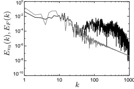
FIGURE 5. Spectra of the time series of the mean velocity (gray line) and integrated Lorentz force (dark line). Only the signals corresponding to the kinematic simulation are considered.
