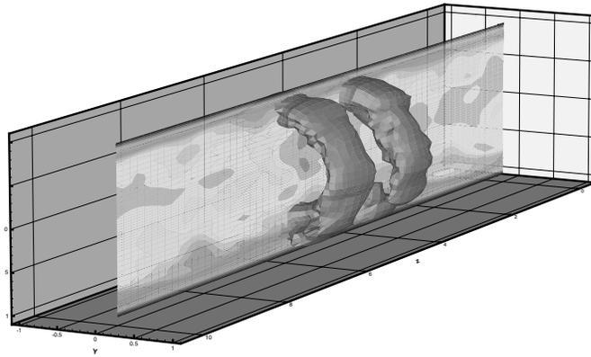
FIGURE 4. Iso-contour of the Lorentz force in the region of space where it is the strongest. The sliced plane contains a contour of the intensity of the velocity field in the streamwise direction.
