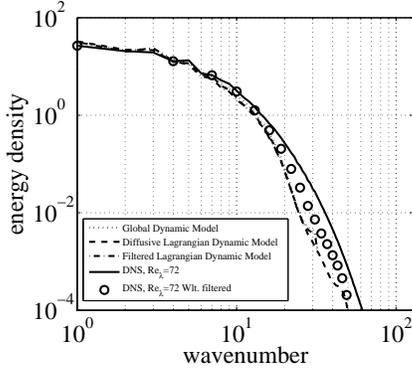
FIGURE 9. Energy density spectra at  $t = 0.16$  for DNS (—), filtered DNS ( $\circ$ ), SCALES with Lagrangian path-line diffusive averaging model (----), filtered Lagrangian path-tube averaging model (-·-·-), and global dynamic Smagorinsky model (·····).
