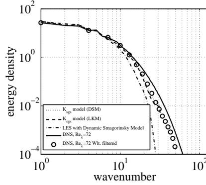
FIGURE 10. Energy density spectra at  $t = 0.16$  for DNS (—), filtered DNS ( $\circ$ ), SCALES with dynamic structure model (·····), localized eddy-viscosity model (----), and LES with global dynamic Smagorinsky model (-·-·-).
