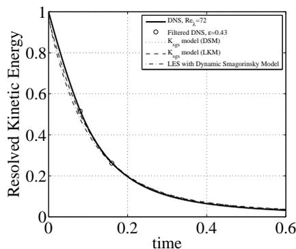
FIGURE 2. Energy decay for SCALES with dynamic structure model (·····), localized eddy-viscosity model (-----), LES with global dynamic Smagorinsky model (-·-·-·), and for comparison DNS (——). Wavelet filtered DNS is shown for 2 stations at which energy spectra will be presented below (o).
