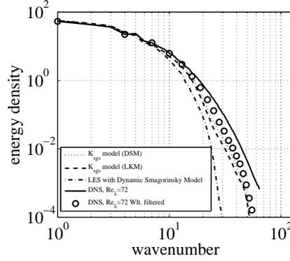
FIGURE 8. Energy density spectra at  $t = 0.08$  for DNS (—), filtered DNS ( $\circ$ ), SCALES with dynamic structure model (·····), localized eddy-viscosity model (----), and LES with global dynamic Smagorinsky model (-·-·-).
