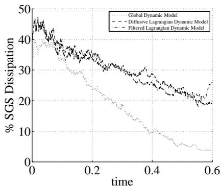
FIGURE 5. Percentage of SGS (modeled) dissipation for SCALES with Lagrangian path-line diffusive averaging model (-----), filtered Lagrangian path-tube averaging model (-·-·-·), and global dynamic Smagorinsky model (·····).
