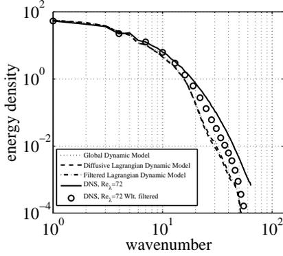
FIGURE 7. Energy density spectra at  $t = 0.08$  for DNS (—), filtered DNS ( $\circ$ ), SCALES with Lagrangian path-line diffusive averaging model (----), filtered Lagrangian path-tube averaging model (-·-·-), and global dynamic Smagorinsky model (·····).
