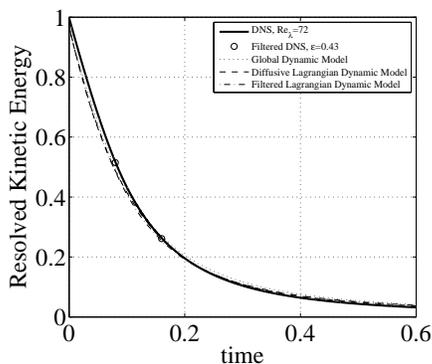
FIGURE 1. Energy decay for SCALES with Lagrangian path-line diffusive averaging model (-----), filtered Lagrangian path-tube averaging model (-·-·-·), global dynamic Smagorinsky model (·····), and for comparison DNS (——). Wavelet filtered DNS is shown for 2 stations at which energy spectra will be presented below (o).
