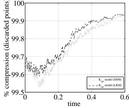
FIGURE 4. Field compression for SCALES with dynamic structure model (·····), localized eddy-viscosity model (-----). For comparison, the compression for LES with global dynamic Smagorinsky model was 98.4%.
