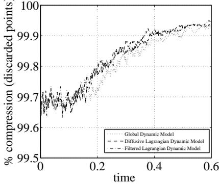
FIGURE 3. Field compression for SCALES with Lagrangian path-line diffusive averaging model (-----), filtered Lagrangian path-tube averaging model (-·-·-·), and global dynamic Smagorinsky model (·····).
