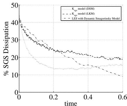
FIGURE 6. Percentage of SGS (modeled) dissipation for SCALES with dynamic structure model (·····), localized eddy-viscosity model (-----), and LES with global dynamic Smagorinsky model (-·-·-·).
