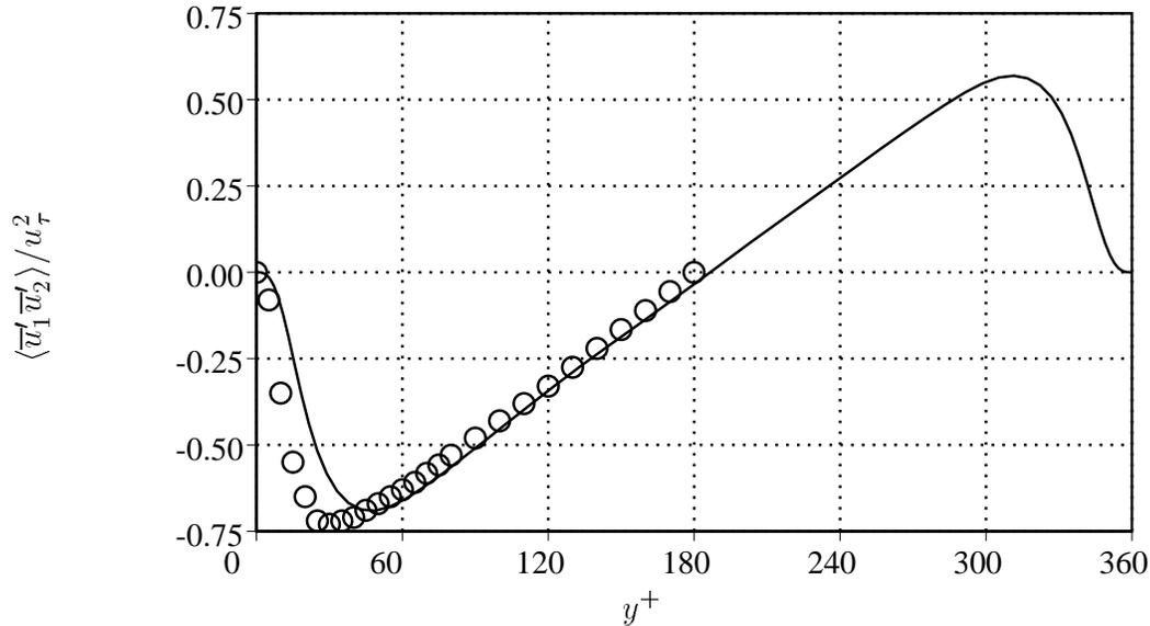
FIGURE 8. Turbulence shear stress normalized by the square of the wall friction velocity for the planar channel flow at  $Re_\tau = 180$ . Symbols ( $\circ$ ) are the DNS data of Kim *et al.* (1987). Lines (—) are computations using the Lagrangian dynamic Smagorinsky model (resolved portion).
