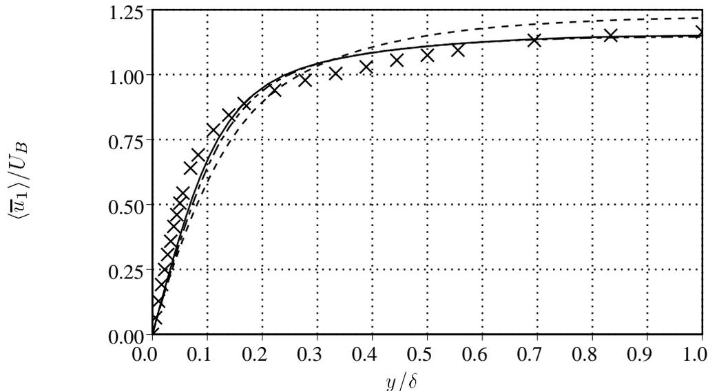
FIGURE 5. Streamwise mean velocity profiles normalized by the bulk velocity  $U_B$  for the planar channel flow at  $Re_\tau = 180$ . Symbols ( $\times$ ) are the DNS data of Kim *et al.* (1987). Lines are computations on the  $33 \times 65 \times 33$  mesh: ---- constant-coefficient Smagorinsky,  $C_s = 0.17^2$ ; -·-·- dynamic Smagorinsky; — Lagrangian dynamic Smagorinsky.
