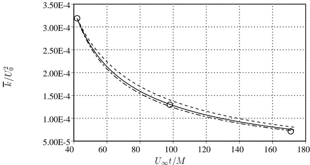
FIGURE 1. Decay of filtered turbulence kinetic energy for homogeneous isotropic decaying turbulence. Filter corresponds to a top-hat in physical space on a  $32^3$  uniform mesh with trapezoidal-rule integration. Symbols are measurements of Comte-Bellot & Corrsin (1971):  $\circ$ . Lines are computations: ---- no subgrid-scale model; -.- constant-coefficient Smagorinsky model with  $C_s = 0.17^2$ ; — dynamic Smagorinsky model.
