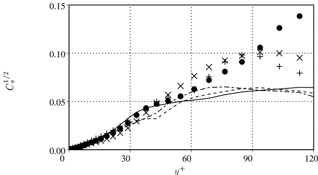
FIGURE 6. Computed profiles of  $C_s^{1/2}$  adjacent to the lower wall for the planar channel flow at  $Re_\tau = 180$ . Symbols ( $\bullet$ ,  $\times$ ,  $+$ ) are planar-averaged profiles from the dynamic Smagorinsky model at three instants of time. Lines (—, ---, - - -) are planar-averaged profiles from the Lagrangian dynamic Smagorinsky model at three instants of time.
