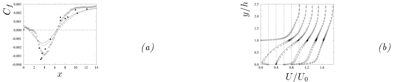
FIGURE 2. (a) Friction coefficient, \circ DNS (Le & Moin), \blacktriangle experiment (Jovic & Driver), \text{—} SMC, \text{---} modified SMC (cf. section 5), (b) DNS U-profiles at locations x/h = -3 ( \circ ), 4 ( \square ), 6 ( \diamond ), 10 ( \triangle ), 15 ( \triangleleft ) and 19 ( \nabla ), \text{—} : model.
