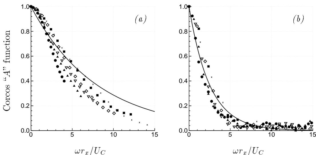
FIGURE 2. Streamwise coherence in Corcos similarity form. (a) Zero pressure gradient flow for selected values of frequency  $\omega$ : ● 0.31, ▲ 0.47, ▽ 0.63, ◇ 0.79, ■ 0.94, × 1.1; ———  $e^{-0.125\omega r_x / U_C}$ . (b) Adverse pressure gradient flow at  $x = 120$ ;  $\omega =$  ● 0.21, ▲ 0.31, ▽ 0.42, ◇ 0.52, ■ 0.63, × 0.73; ———  $e^{-0.4\omega r_x / U_C}$ .
