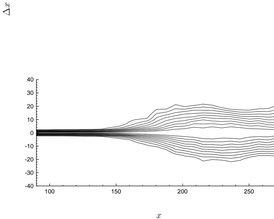
FIGURE 6. Wall pressure two-point streamwise separation correlation contours.
