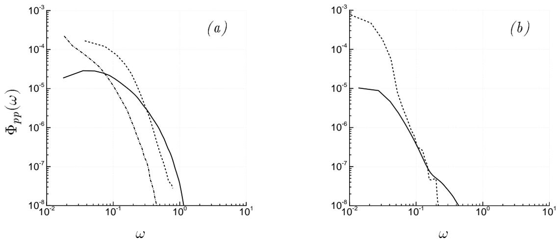
FIGURE 10. Wall pressure frequency spectrum. (a)  $x = 160$ ; — model (Eq. 4 using velocity spectrum at  $y = 7.07$ ), -·- model (Eq. 4 using velocity spectrum at  $y \approx 2.28$ ), ---- DNS. (b)  $x = 220$ ; — model (Eq. 4), ---- DNS.
