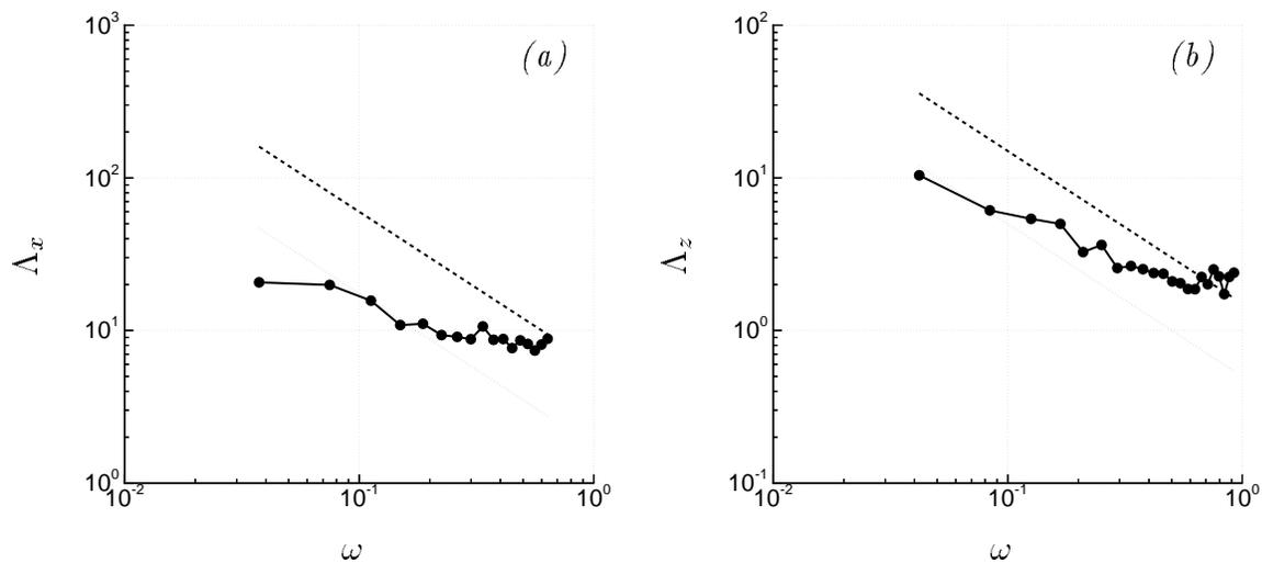
FIGURE 4. (a) Streamwise coherence length scales:  $\bullet$  DNS,  $\cdots$   $1.75U/\omega$ ,  $---$   $6.0/\omega$ . (b) Spanwise coherence length scales:  $\bullet$  DNS,  $\cdots$   $1.5U/\omega$ ,  $---$   $0.5U/\omega$ .
