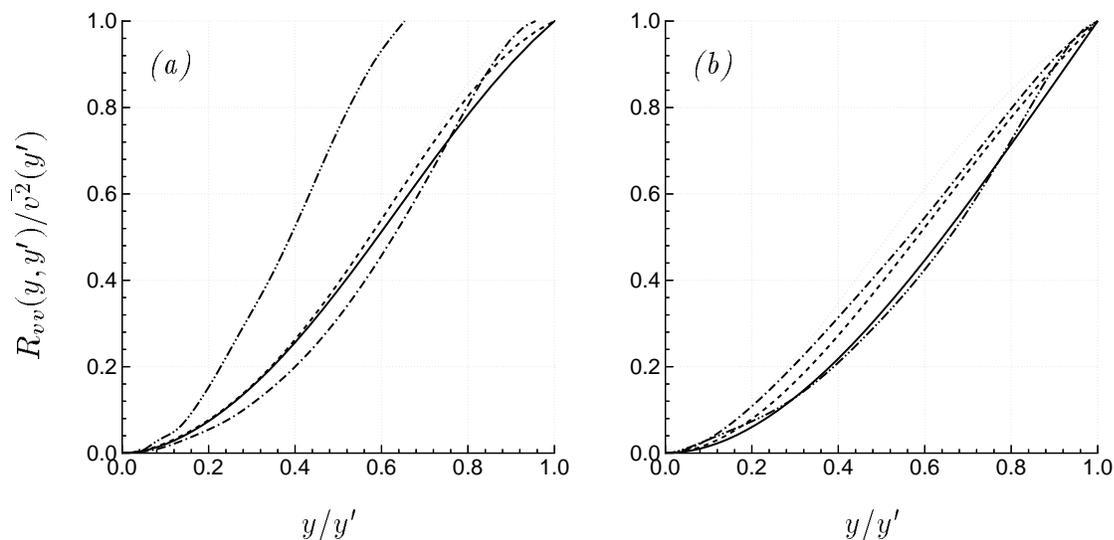
FIGURE 5. Two-point correlation of wall-normal velocity component, (a)  $x = 80$ , (b)  $x = 220$ ;  $—$   $y' = 0.5$ ,  $---$   $y' = 1.0$ ,  $\cdots$   $y' = 2.0$ ,  $- \cdot -$   $y' = 4.0$ ,  $- - -$   $y' = 8.0$ .
