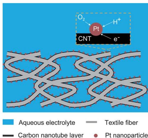
**Fig. 1** Schematic of the CNT–textile–Pt composite in aqueous electrolyte. While the electrochemical deposition method guarantees electronic access to the Pt, the open and macroscale porous structure of the CNT–textile facilitates the contact between the Pt and the aqueous electrolyte containing oxygen.
