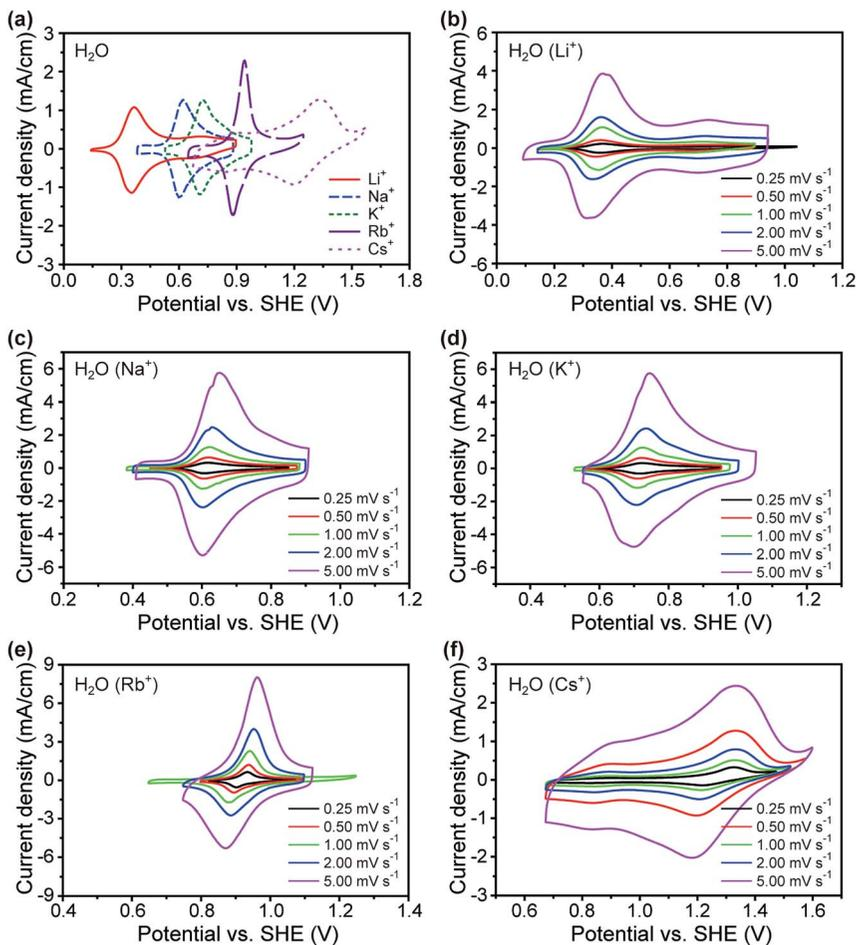
Fig. 5 CV curves of NiHCFE using the three-electrode Swagelok cell configuration in aqueous electrolytes. The scan rate is  $1 \text{ mV s}^{-1}$ . (a) CV curves of  $\text{Li}^+$ ,  $\text{Na}^+$ ,  $\text{K}^+$ ,  $\text{Rb}^+$ , and  $\text{Cs}^+$  ions. CV curves of (b)  $\text{Li}^+$ , (c)  $\text{Na}^+$ , (d)  $\text{K}^+$ , (e)  $\text{Rb}^+$ , and (f)  $\text{Cs}^+$  ions at different scan rates from 0.25 to  $5.00 \text{ mV s}^{-1}$ .
