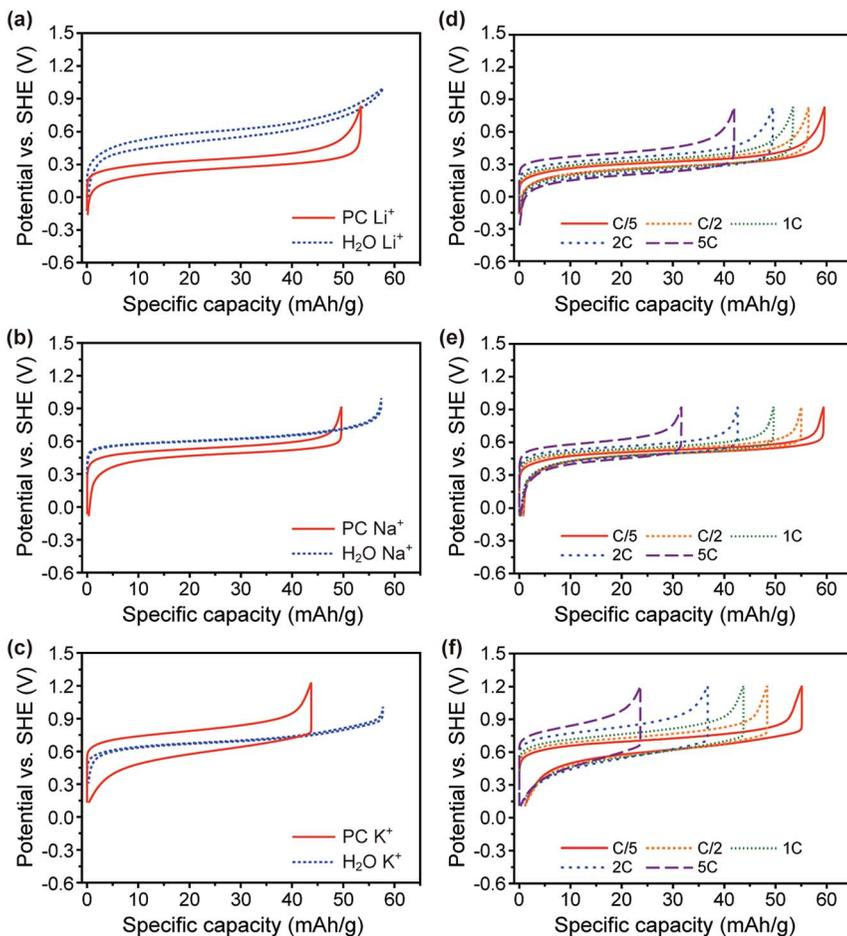
Fig. 3 Comparison of hysteresis in galvanostatic potential profiles at 1 C between aqueous and PC electrolytes. (a) Li<sup>+</sup>, (b) Na<sup>+</sup>, and (c) K<sup>+</sup> ion systems. Typical charge and discharge potential profiles of NiHCFE electrodes at different C rates (0.2, 0.5, 1, 2, and 5 C) with (d) Li<sup>+</sup>, (e) Na<sup>+</sup>, and (f) K<sup>+</sup> ions in PC.
