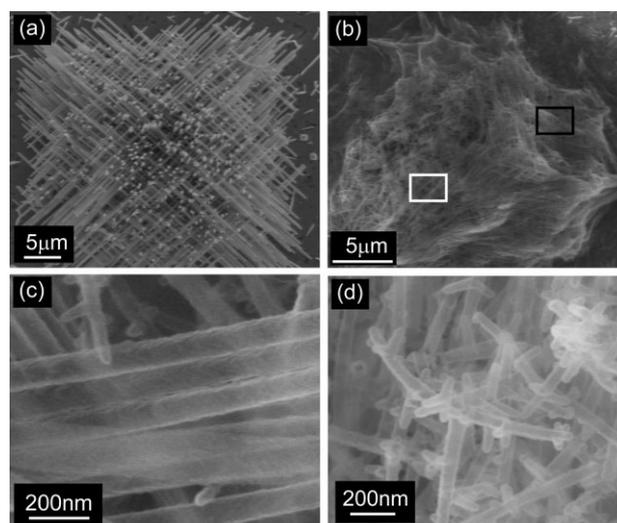
Figure 2. a) An SEM image of PbSe hyperbranched nanowire coated with 30-nm  $\text{SiO}_2$ . (b) Interconnected  $\text{SiO}_2$  nanotubes with a 30-nm-thick shell. (c) and (d) High resolution SEM images of interconnected  $\text{SiO}_2$  tubes taken from white and black box of (b), respectively.
