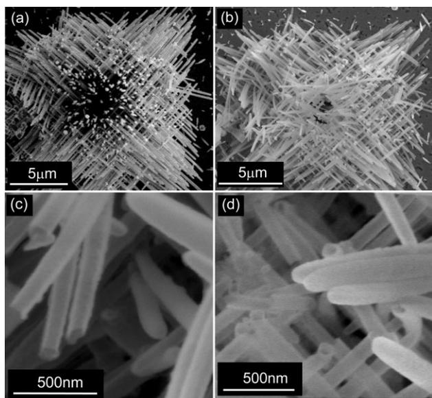
**Figure 3.** a) An SEM image of a hyperbranched PbSe hyperbranched nanowire with 80-nm SiO<sub>2</sub> shell after FIB cut. b) Interconnected SiO<sub>2</sub> nanotubes with 80-nm shell and after aqua regia etching. c) and d) High resolution SEM images of SiO<sub>2</sub> tubes with open end from (b).
