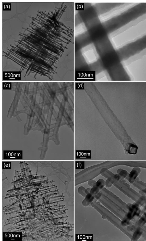
**Figure 4.** a) and b) TEM images of a hyperbranched PbSe hyperbranched nanowire with 30-nm SiO<sub>2</sub> coating. c) A TEM image of hyperbranched nanotubes with an 30-nm-thick silica shell. d) A TEM image of silica nanotube with open end. e) and f) TEM images of nanotubes network with an 80-nm-thick silica shell.
