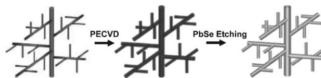
Figure 1. Flowchart of the fabrication process for interconnected silica nanotubes from hyperbranched PbSe nanowires.
