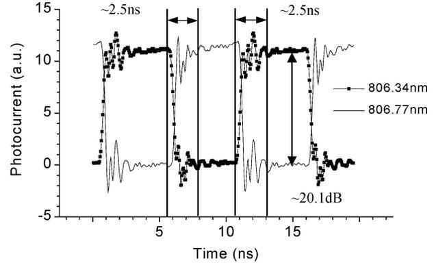
Fig. 6. Photocurrent output of the device as the biasing pattern is changed to select one wavelength or the other. The biasing pattern applied on the device alternates every 5 ns to select between 806.34 and 806.77 nm. The device wavelength switching access time is  $\sim 2.5$  ns and the ON/OFF contrast ratio for selecting one wavelength while deactivating the other is  $\sim 20.1$  dB.
