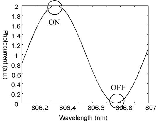
Fig. 4. Simulation of the spectral response of the tunable photodetector enabling 806.34 nm and disabling 806.77 nm. The optical path length difference between the two interfered beams is  $\sim 0.763$  mm.
