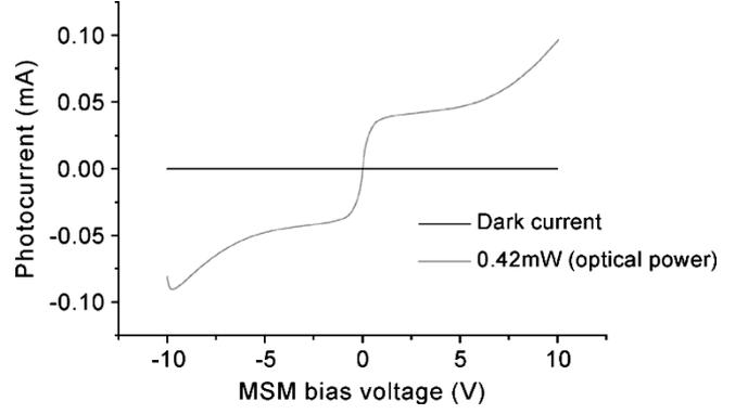
Fig. 2. Photocurrent response of an MSM diode with and without optical power.
