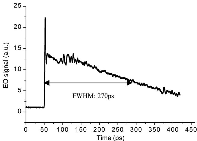
Fig. 8. Intrinsic response of the tunable photodetector measured with a subpicosecond optical input pulse and electrooptic sampling of the output, with 1.65-V bias.
