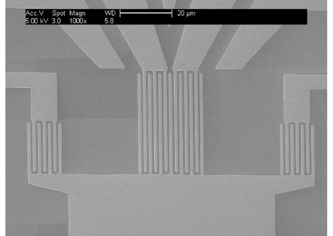
Fig. 5. Scanning electron microscopy photograph of the fabricated tunable photodetector with  $1 \mu\text{m}$  finger spacing and width. The pattern in the center region of the device is used to perform wavelength switching, while the fingers in the left region are used for adjusting the spectral response to achieve a good wavelength-selective contrast ratio. The right region is a dummy structure for symmetry of the device.
