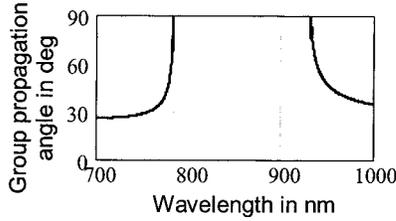
Fig. 2. Group-propagation angle as a function of wavelength for an infinite 1-D photonic crystal consisting of alternating 167 nm  $\text{SiO}_2$  ( $n=1.46$  at 830 nm) and 110 nm  $\text{Ta}_2\text{O}_5$  ( $n=2.06$ ) layers at  $\theta_{\text{in}}=45^\circ$  and of  $p$  polarization calculated by Bloch theory.
