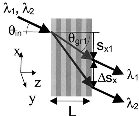
Fig. 1. Superprism effect in a 1-D photonic crystal.
