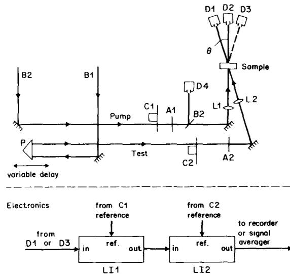
Fig. 4. Schematic of the experimental setup. The laser beams  $B1$  and  $B2$  originate either from a dye laser or from a diode laser. The test beam can be delayed with respect to the pump beam. Detectors  $D1$ – $D4$  are silicon photodiodes, choppers  $C1$  and  $C2$  provide the references for lock-in amplifier signal processing [5].  $A1$  and  $A2$  are neutral density filters. Depending on the beam angle  $\theta$ , one or two lenses are used to focus the beams on the sample.
