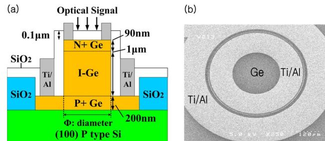
Fig. 1. (a) Schematic diagram of the cross section of normal incidence Ge/Si p-i-n photodiode. (b) Scanning electron micrograph of the circular mesas of the photodiodes. The circular p-i-n device has the ring-shaped contact with a ring width of 50  $\mu\text{m}$ .
