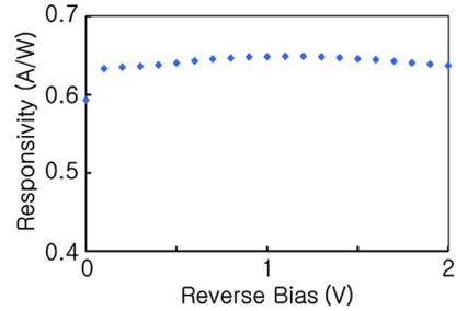
Fig. 3. Photodetector responsivity at  $\lambda = 1.55 \mu\text{m}$  versus reverse bias for the mesa Ge p-i-n photodiodes with a radius of 100  $\mu\text{m}$ .
