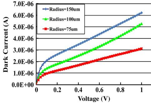
Fig. 2. Dark current versus reverse-bias curves of the circular-shaped mesa Ge/Si p-i-n photodiodes.
