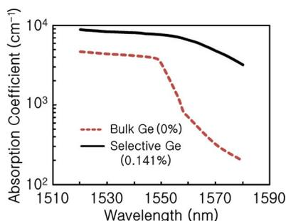
Fig. 4. Absorption coefficient at 2-V reverse-bias versus photon wavelength. The absorption coefficient ( $\alpha$ ) is extracted from the measured responsivity, assuming 90% internal efficiency. The  $\alpha$  for bulk Ge is plotted for reference.
