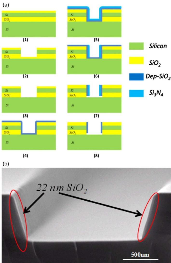
Fig. 4. (a) Process flow for the thin spacer fabrication process. (b) Fabrication results: 22 nm SiO<sub>2</sub> on sidewalls with 80° slope of a growth window trench.
