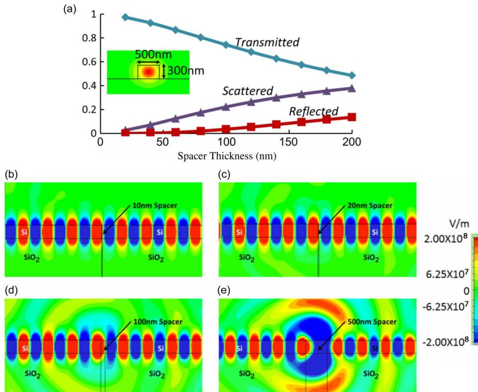
Fig. 3. (a) Percentages of transmitted, scattered, and reflected optical power for different spacer thicknesses. (Inset) Mode profile of the fundamental quasi-TE mode for a 500-nm-wide and 300-nm-thick SOI waveguide. (b)–(e) Electric field distribution for different spacer thicknesses in the cross sectional plane along the dashed line in Fig. 2(a).
