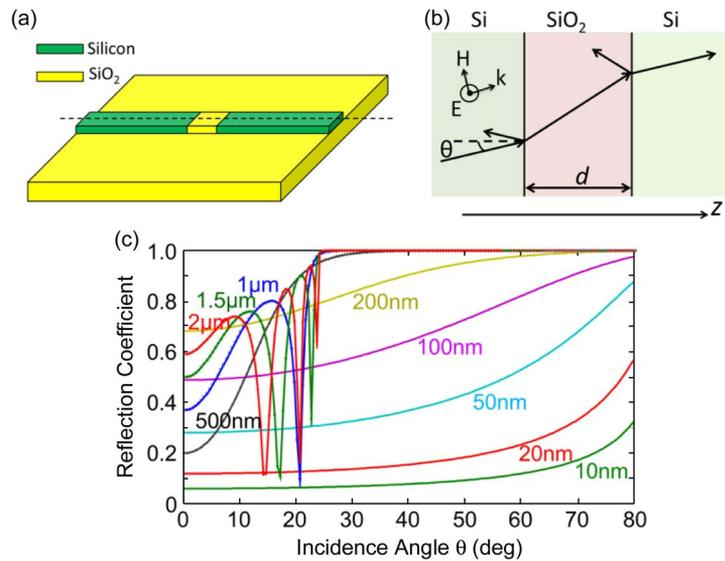
Fig. 2. (a) Schematic of the problem setup. Propagation through two SOI waveguide sections with a SiO<sub>2</sub> spacer in between. (b) Simplified 1-D model for a plane wave component with incidence angle  $\theta$ . (c) Electric field reflection coefficient evaluated for various angles with different spacer thicknesses.
