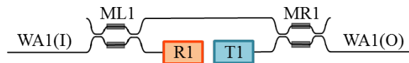
Fig. 3. Bypass switching. Additional waveguide switches, here implemented using MZIs ML1 and MR1, can be used to connect waveguide WA1(I) directly to WA1(O), bypassing the receiver R1 and transmitter T1.
