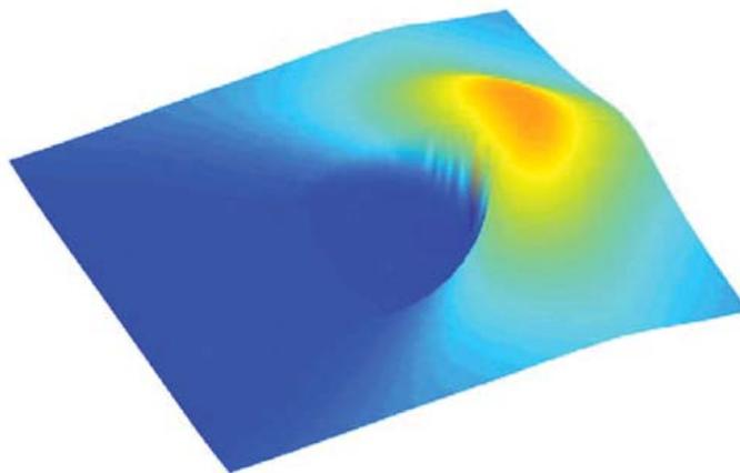
**Figure 2.** Simulation of a pulse just after it has passed 'through' (from left to right) a 'truly cloaked' spherical volume. Height and false color represent the pulse amplitude in the equatorial plane.
