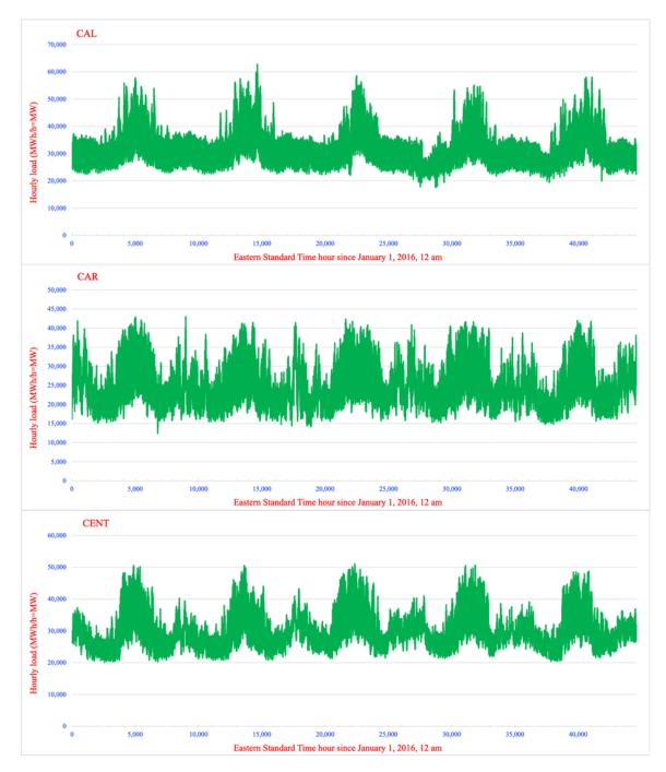
**Figure S1.** Unmodified 2016-2020 hourly electric load (MWh/h=MW) for each of the load regions listed in Table S1, which also shows the annual average load for each region each year. Data are from EIA (2021a).
