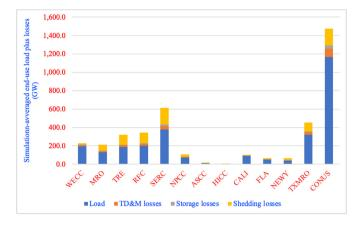
**Fig. 4.** Shares (GW) of simulation-averaged power produced by WWS used to meet end-use load, transmission, distribution, and maintenance (TD&M) losses, losses in and out of storage, and shedding losses. Table S15 provides exact values used in the figure. Table 2 defines the regions.
