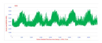
Fig. 1. Unmodified 2016–2020 hourly electric load (MWh/h = MW) for the Texas region [45]. Table S1 shows the average load by year.
