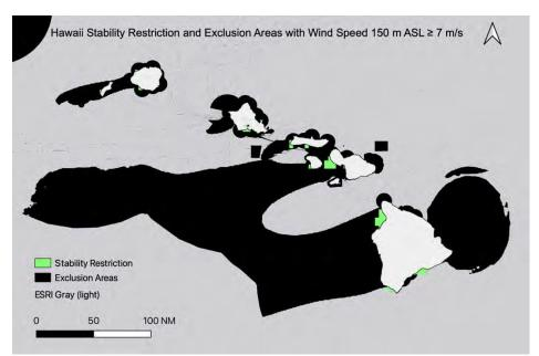
**Figure S6.5:** Hawaii Stability Restriction (green) after accounting for all restrictions plus 150 m ASL  $\geq$  7 m/s wind speed threshold (see Table S1 for details about each restriction layer). 718,462 km<sup>2</sup> (60.6%) of total Hawaii area would be available for wind turbine development using a 30% stability threshold. There is a 0.023% difference in available area when restricting stability versus not.
