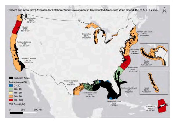
Fig. 2. Percent and Area (km²) Available for Offshore Wind Development. Map shows the percentage and offshore area available for wind farms after excluding all restrictions in Table S1 and wind speeds below 7 m/s at 150 m ASL. Colors indicate the percentage of available area in each of the fifteen study regions. See Tables S3-4 for all hub height and wind speed threshold combinations.
