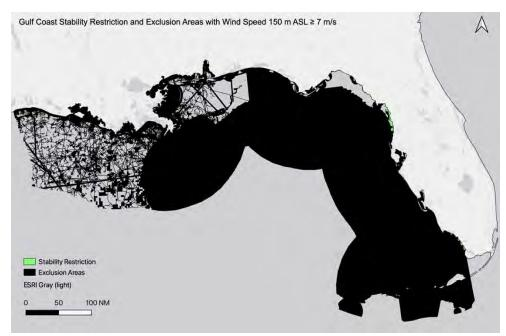
**Figure S6.3:** Gulf Coast Stability Restriction (green) after accounting for all restrictions plus 150 m  $ASL \ge 7$  m/s wind speed threshold (see Table S1 for details about each restriction layer). 137,675 km<sup>2</sup> (28.6%) of total Gulf Coast area would be available for wind turbine development using a 30% stability threshold. There is a 0.09% difference in available area when restricting stability versus not.
