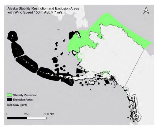
**Figure S6.4:** Alaska Stability Restriction (green) after accounting for all restrictions plus 150 m ASL ≥ 7 m/s wind speed threshold (see Table S1 for details about each restriction layer). 1,398,720 km<sup>2</sup> (56.4%) of total Alaska area would be available for wind turbine development using a 30% stability threshold. There is a 27.6% difference in available area when restricting stability versus not.
