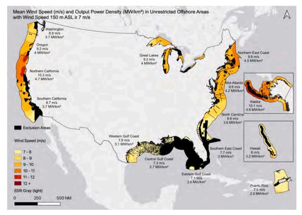
Fig. 5. Mean Wind Speed (m/s) and Output Power Density (MW/km²). The mean wind speed in each region is shown alongside the output power density (MW/km²) in all unrestricted offshore areas with wind speed at 150 m ASL  $\geq$  7 m/s. The color scale represents the full range of wind speed values (m/s) in each grid cell. See Figs. S5.1–5.4 and Table S8 for all hub height and wind speed threshold combinations.
