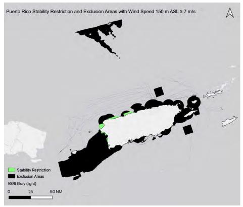
**Figure S6.6:** Puerto Rico Stability Restriction (green) after accounting for all restrictions plus 150 m  $ASL \ge 7$  m/s wind speed threshold (see Table S1 for details about each restriction layer). 104,102 km<sup>2</sup> (88.6%) of total Puerto Rico area would be available for wind turbine development using a 30% stability threshold. There is a 0.053% difference in available area when restricting stability versus not.
