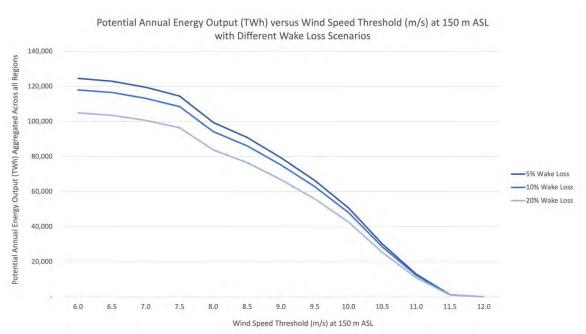
**Figure S2.2: Potential Annual Energy Output (TWh) versus Wind Speed Threshold (m/s).** Graph shows how cumulative energy output at 150 m ASL varies with wind speed thresholds for different wake loss scenarios (dark blue: 5%, medium blue: 10%, light blue: 20%). Not shown is no wake loss scenario. See Tables S11-12 for all hub height and wake loss combinations.
