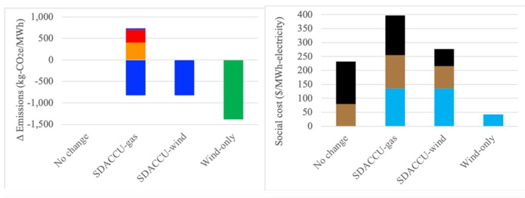
No change: coal and no SDACCU; SDACCU-gas: coal and SDACCU powered by gas; SDACCU-wind: coal and SDACCU powered by wind; Wind-only: Coal replaced by wind and no SDACCU
