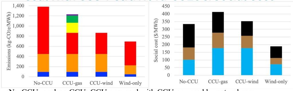
No-CCU: coal-no CCU; CCU-gas: coal with CCU powered by natural gas; CCU-wind: Coal-CCU powered by wind; Wind-only: replace coal with wind Blue=upstream coal non-CH<sub>4</sub> CO<sub>2</sub>e; Orange=coal upstream CH<sub>4</sub> CO<sub>2</sub>e; Red=coal CO<sub>2</sub>; Yellow=Gas CO<sub>2</sub>; green=Gas CO<sub>2</sub>e from CH<sub>4</sub> leaks; Purple=other gas upstream CO<sub>2</sub>e; Light blue=electricity+CCU cost; Brown=air pollution cost; Black=climate cost
