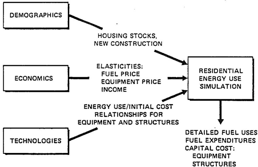
Figure 3-12 Schematic of Hirst Residential Energy-Use Model
