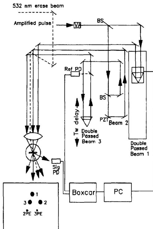
Fig. 1. Apparatus used to perform two-pulse photon and three-pulse stimulated echoes. VA=variable attenuator, BS=beam-splitter, PZT=piezo-electric transducer, PD=photodiode. The inset shows the location of the signals relative to the input beams.
