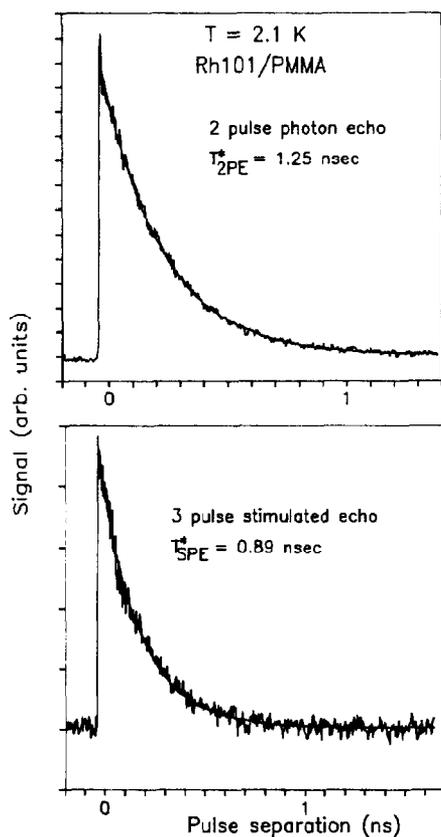
Fig. 2. Comparison of two-pulse photon echo ( $T_w=0$ ) and three-pulse stimulated echo ( $T_w=2$  ns) in Rh101/PMMA at 2.1 K. The stimulated echo is approximately 35% faster than the two-pulse echo as a result of spectral diffusion in the polymer glass. The solid lines are fits to an exponential.
