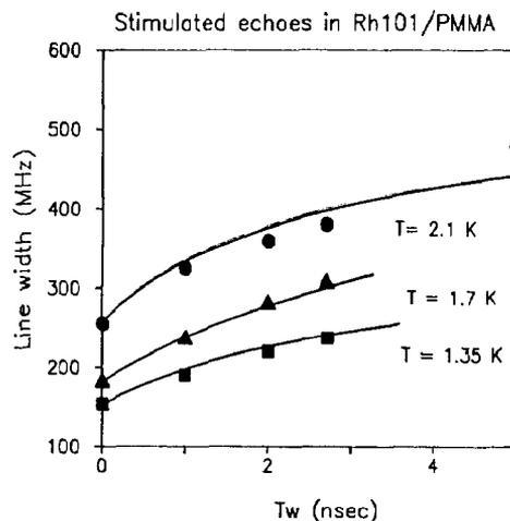
Fig. 3. Temperature- and waiting-time-dependent study of two- and three-pulse echoes in Rh101/PMMA. The decay times are plotted as lifetime corrected line widths (see text). Line widths increase with temperature and  $T_w$ . The solid lines are predicted values for the line widths based on an analysis of the stimulated echo correlation function for short waiting times.
