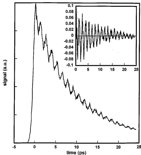
FIG. 3. Vibrational echo data on H64V in glycerol–water at 3.4 K with the laser tuned to  $1957\text{ cm}^{-1}$ . The center of the  $\nu=0\rightarrow 1$  transition for this line is  $1969\text{ cm}^{-1}$ . The excitation bandwidth was  $\sim 16\text{ cm}^{-1}$  FWHM. The dephasing times of the  $\nu=1\rightarrow 2$  and  $\nu=0\rightarrow 1$  transitions are 20 and 65 ps, respectively.
