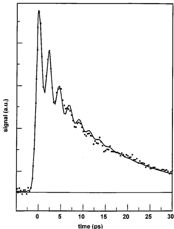
FIG. 4. Vibrational echo decay and fit  $\text{W}(\text{CO})_6$  in dibutylphthalate at 10 K and  $1976.3 \text{ cm}^{-1}$ . The beats are separated by 2.3 ps, corresponding to a vibrational anharmonic splitting of  $\Delta = 14.7 \text{ cm}^{-1} \pm 0.3 \text{ cm}^{-1}$ .
