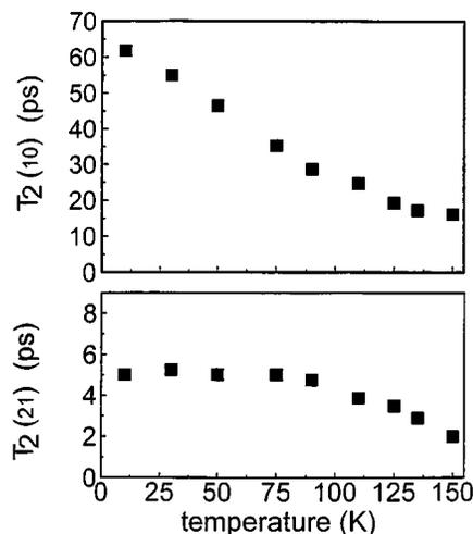
FIG. 5. Decay times  $T_2(01) = 1/\gamma_{01}$  and  $T_2(12) = 1/\gamma_{12}$  of  $\text{W}(\text{CO})_6$  in DBP for temperatures between 10 and 150 K obtained from fits to Eq. (3). The lack of temperature dependence of  $T_2(12)$  at the lower temperatures shows that  $T_2$  is lifetime limited.
