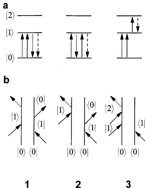
FIG. 6. (a) Ladder diagram of the three pulse sequences in a VEB experiment. The first two diagrams are the two-level vibrational echo diagrams. The solid arrows denote interactions on the ket of the density matrix, while dotted arrows denote interactions on the bra of the density matrix. The signal is indicated with the dashed arrows. (b) Another representation of the three pulse sequences of in the VEB experiment. Time is taken to increase moving up the parallel set of lines.
