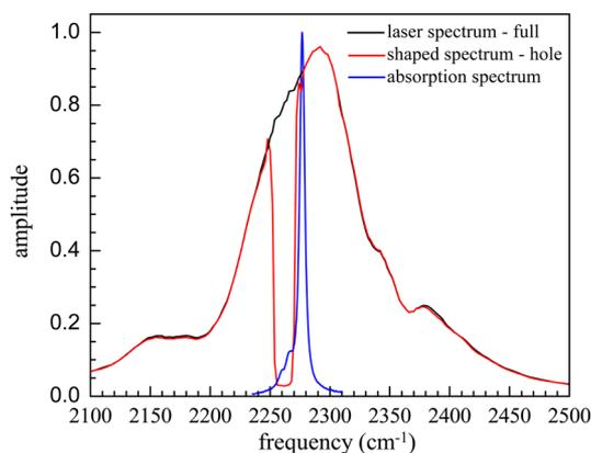
**Figure 6.** Spectrum of the full pump laser pulse (black curve) and the spectrum of the pulse with a hole in the frequency distribution (red curve) that eliminates pumping of the hot band. The absorption spectrum of the  $^{13}\text{CO}_2$  asymmetric stretch (blue curve) is superimposed for comparison.
