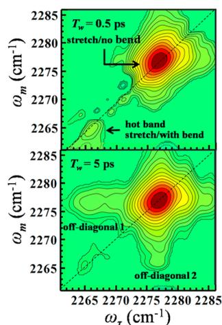
**Figure 4.** Two-dimensional infrared (2D IR) spectra of  $^{13}\text{CO}_2$  in EmimNTf<sub>2</sub> at two waiting times,  $T_w = 0.5$  and 5 ps. The dashed lines are the diagonals. Off-diagonal peaks grow in by the longer waiting time. The growth of the off-diagonal confirms the transfer of population from the hot band to the main band and vice versa. Contour lines are on a logarithmic scale to better visualize the small peaks.
