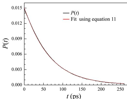
**Figure 5.** Population relaxation,  $P(t)$ , data (black curve) measured at the asymmetric stretch absorption peak frequency ( $2277 \text{ cm}^{-1}$ ), along with the corresponding fit (red curve) to the kinetic model (eq 11). The fit has only two adjustable parameters,  $\tau_b$ , the bend lifetime and an overall normalization constant. The stretch lifetime was obtained from the single exponential fit at long times (see Figure 3).
