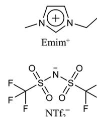
**Figure 1.** Structure of the ionic liquid used: 1-ethyl-3-methylimidazolium bis(trifluoromethylsulfonyl)imide, abbreviated as EmimNTf<sub>2</sub> throughout the paper.
