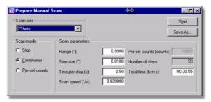
Select "2Theta" from the "Scan axis" drop-down list. In the "Scan mode" box select the "Continuous" radio button and the following parameters:
