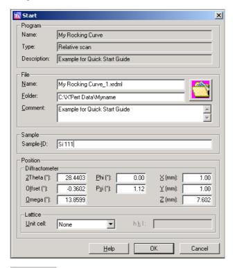
Press OK After a while the scan window will appear and shortly afterwards, your rocking curve measurement will be completed, at which time the goniometer will return to its rest positions.
