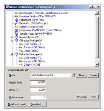
Confirm that the information displayed here is correct for all diffracted beam paths (in this example: two). Press the Next button to see the "Axes" frame containing the limits and rest positions which we will not change at this time.
