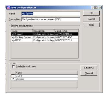
• If you have more than one sample stage you should make a configuration for each sample stage. In order to do that you must mount each of your sample stages in turn and then create a configuration for that stage by repeating the actions in this section (3.4.1). Exchanging sample stages is described in Chapter 5, section 5.4.1.
