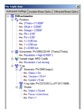
Double-click on the "Generator" branch to open the Instrument Settings window at the X-ray tab. Enter the required values (in this example: "45 kV" and "40 mA").
