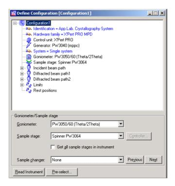
If you have more than one sample stage available to you, check the "Get all sample stages in instrument" check box in order to reduce the number of sample stages in the drop-down list of sample stages to only those available. Press the button to see the Incident Beam Path description.
