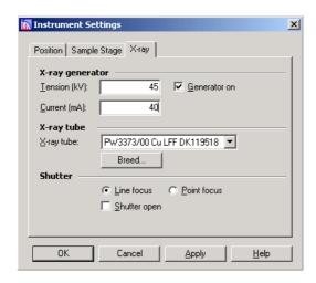
**Note:** If you have a PSD you should select a lower value (for example: "35 kV" and "30 mA") to avoid saturating the detector.
