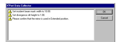
Carry out the requested actions and then press OK. The incident beam optics reflect the actual situation.
