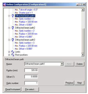
As this configuration only uses the beam path that we removed in section 4.4.1 we must now remove the other two beam paths from the configuration (in this example: Diffracted beam path 1 and Diffracted beam path 2).
