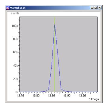
If necessary, go back to Move mode and move the hairline into the middle of the peak.
