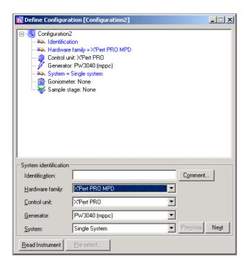
Find out what hardware is known to the instrument control software by pressing Read Instrument. Wait until the system is ready (the "Connecting to instrument" pop-up disappears).
