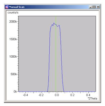
Make a note of the count rate at the peak. You can see that by moving the + cursor to the top of the peak and reading the count rate in the status bar (approximately 14 400 in this example).
