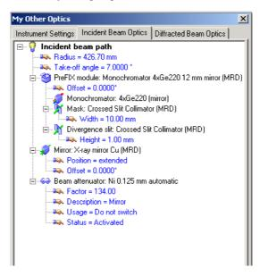
If you are using an uncalibrated beam attenuator you should calibrate the attenuation factor before you continue, if you have a calibrated one, go to section 4.6.4. An uncalibrated beam attenuator shows a beam attenuation factor of 20.00.
