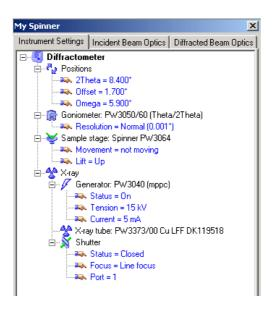
• In the instrument control window double-click on the "Generator" path of the tree and enter "45 kV" and "40 mA":
