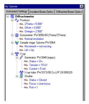
Double-click on "Generator", set the power to "45 kV" and "40 mA".
