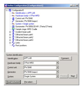
The next step is to set up two new configurations one with two beam paths, and the other with one beam path; in other words tell the computer what the system "looks" like.
