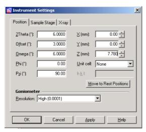
Mount the Z-position dial gauge (to be used as a pointer to the middle of the sample), ensure that Z (mm) = 0 to avoid damaging the sample. Vary the X and Y mm settings until the pointer is over the centre of the sample. To change the positions: enter the new value and press
