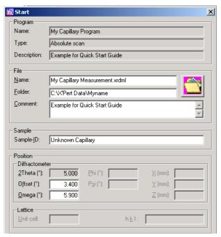
Make sure that the capillary spinner is switched On and that the enclosure doors are closed and then press OK.
