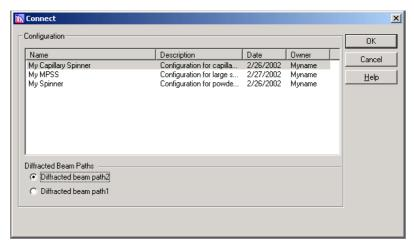
If applicable - select the diffracted beam path with the Bragg-Brentano type optics (in this example: Diffracted beam path 1) and press
