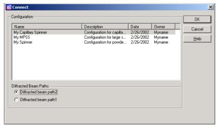
Choose the configuration you want to use (in this example: "My Capillary Spinner") and the beam path containing the X'Celerator (in this example: "Diffracted beam path 2") and press OK . You may be asked to make some changes, if so, make the changes and confirm with
