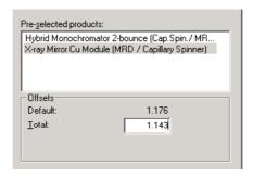
If your system includes an X'Celerator detector (and an X'Celerator detector monochromator) it is important that define the detector offsets provided in the System Acceptance Form delivered with your system.
