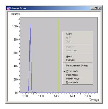
Use the left mouse button to "grab" the hairline, drag it to the centre of the peak and release it. The goniometer moves to that angle.
