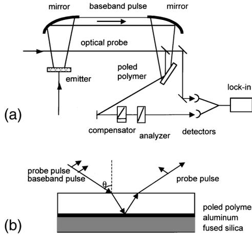
Fig. 1. (a) Schematic diagram of the experimental setup. Ultrashort baseband pulses are generated in  $\langle 110 \rangle$  GaAs and detected in a poled polymer. (b) Expanded view of the poled polymer and beam propagation path. The optical probe and baseband pulses copropagate through the polymer with an external angle of incidence  $\theta$ . The baseband pulse is  $p$  polarized, whereas the optical probe is polarized at  $45^\circ$  with respect to the plane of incidence.
