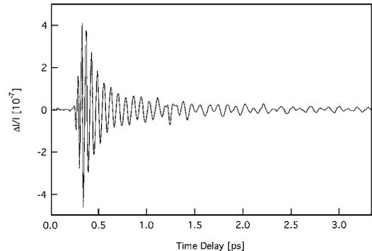
Fig. 2. Temporal waveform detected by electro-optic sampling. The shortest oscillation period is  $\sim 33$  fs.
