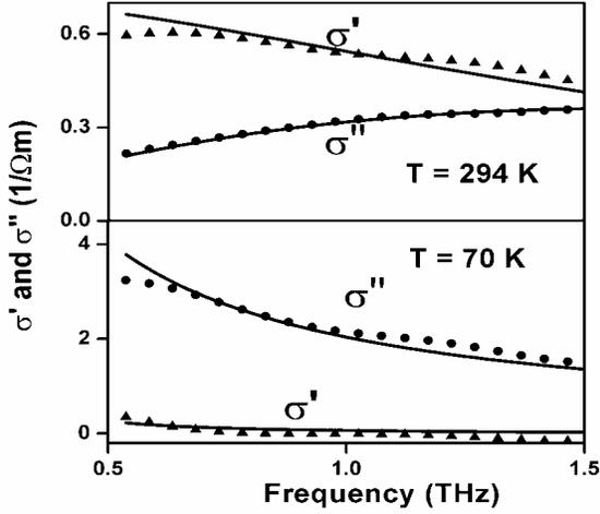
**Fig. 3:** Frequency dependence of the photo-induced complex conductivity for sapphire measured at temperatures of  $294 \text{ K}$  and  $70 \text{ K}$  (symbols). The excitation and probing conditions correspond to those of Fig. 2. The solid lines are fits to the Drude model.
