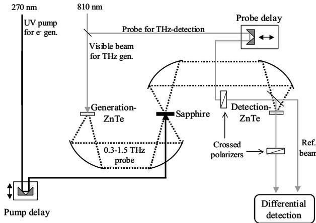
**Fig. 1:** Experimental setup for THz time-domain spectroscopy with a UV pump pulse for the photo-generation of charge carriers. The THz pulses are produced by optical rectification in a ZnTe crystal. Detection of the THz electric field is accomplished by electro-optic sampling with time-synchronized fs laser pulse in a second ZnTe crystal. The sapphire sample is excited with 270 nm radiation generated as the third-harmonic of the mode-locked laser.
