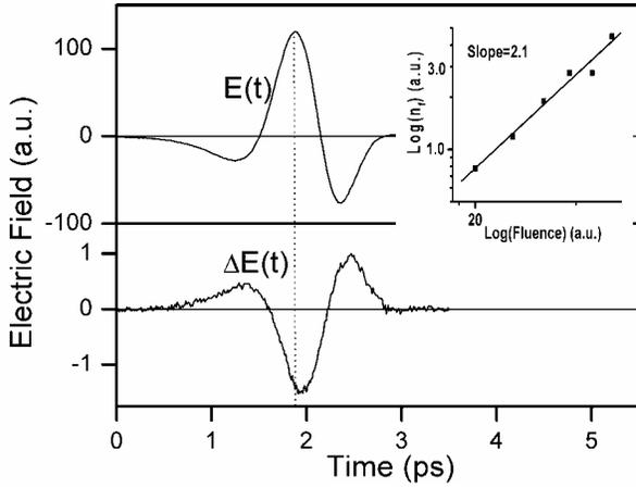
**Fig. 2:** Upper trace: THz electric field,  $E(t)$ , transmitted through a sapphire sample. Lower trace: Photo-induced change in the THz waveform,  $\Delta E(t)$ . The UV pump fluence was  $20 \text{ J/m}^2$  and the pump-probe delay time was  $5 \text{ ps}$ . Inset: log-log plot of the power dependence of the photo-generated response. It is fit to power law with an exponent of 2.1.
