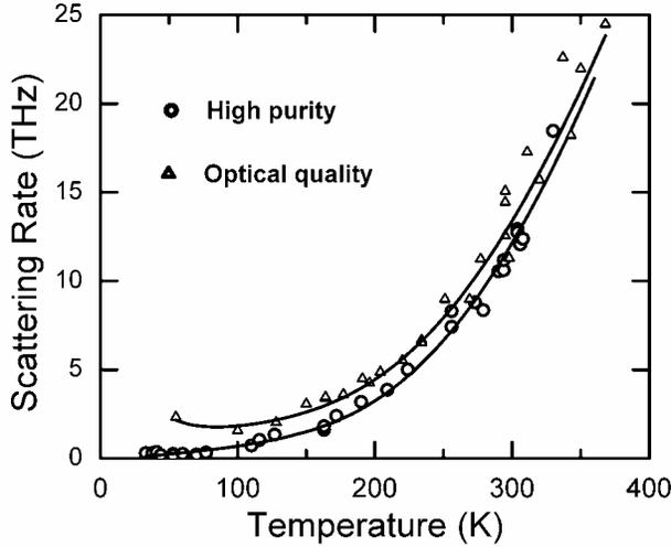
**Fig. 4:** Electron scattering rates in two sapphire crystals of differing purity as a function of temperature, as inferred from a Drude fit to the THz-TDS data. The solid lines are fits to the model described in the text.
