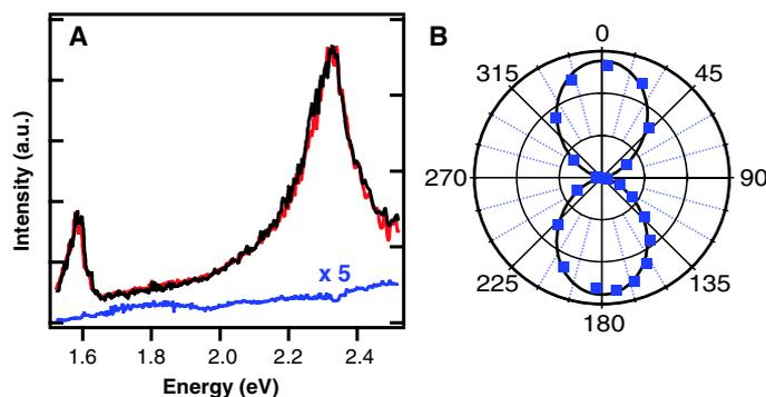
The blue spectrum (magnification  $\times 5$ ) is obtained for incident light polarized perpendicular to the axis of the nanotube. (B) Rayleigh scattering intensity as a function of the angle between the electric field polarization and the tube axis. The solid line is a  $\cos^2 \theta$  fit.
