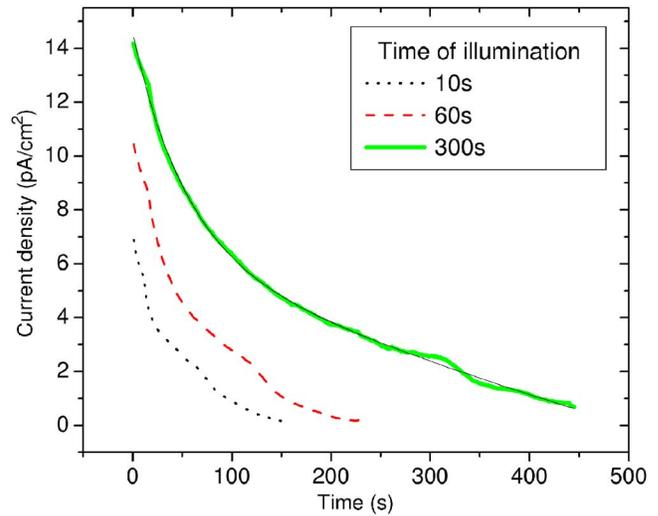
FIG. 4. (Color online) Temporal evolution of the current density after abrupt termination of illumination with broadband radiation for an  $\text{SiO}_2$  film at an applied bias of  $-8 \times 10^5$  V/cm (silicon substrate at positive voltage). Results for three exposure times are shown. The solid black line is a fit for the 300 s data to a decay given as the sum of two exponential functions.
