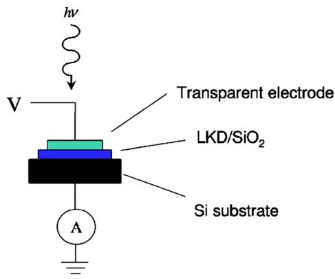
FIG. 1. (Color online) Schematic of layer structure samples, consisting of a silicon substrate, the LKD or  $\text{SiO}_2$  film, and a transparent gold electrode. The light from the mercury lamp, either directly or after being spectrally filtered in a monochromator, is focused on the sample at normal incidence. A bias voltage  $V$  is applied between the gold electrode and the doped silicon substrate, as shown, and the leakage or photoinduced current is recorded.
