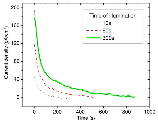
FIG. 5. (Color online) As in Fig. 4, but with a LKD film. Note the longer detrapping time and larger current compared to the behavior for the  $\text{SiO}_2$  film.
