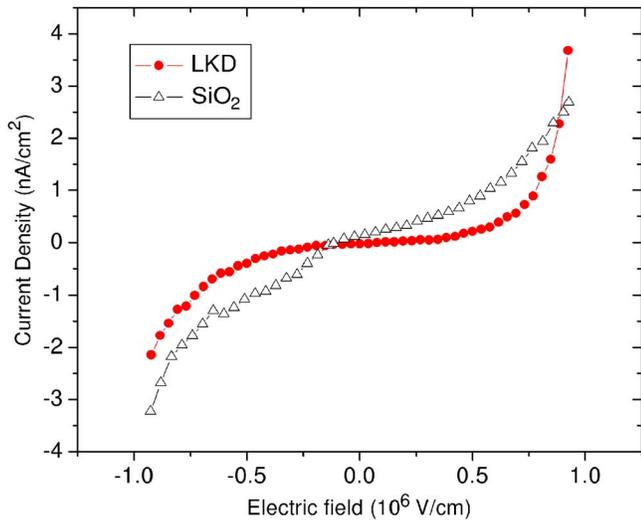
FIG. 3. (Color online) Photoinduced  $I$ - $V$  curves for LKD and  $\text{SiO}_2$  films, plotted as current density vs applied bias electric field. The bias is applied to the gold electrode, with a positive field corresponding to excitation of electrons over the Si/insulator interface and negative fields to excitation across the Au/insulator interface. (The solid lines are guides to the eye.)
