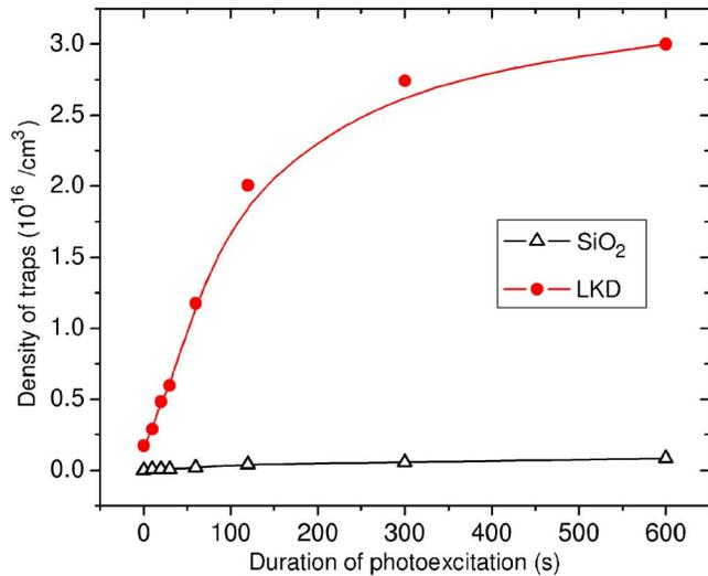
FIG. 6. (Color online) Inferred density of traps in the LKD and SiO<sub>2</sub> films based on the measured charge flow after stopping illumination, as in the data of Figs. 4 and 5. Both SiO<sub>2</sub> and LKD films display an increase in density of filled traps with increasing time of illumination up to a saturated level. (The solid lines are guides to the eye.)
