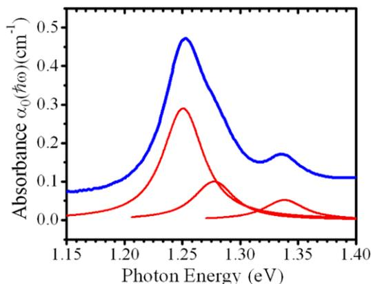
**Fig. 1** Absorption spectrum  $\alpha_0(\hbar\omega)$  of (6,5)-enriched solution of SWNTs as a function of photon energy (blue curve). The peak centered at 1.253 eV arises from the  $E_{11}$  excitonic transitions of (6,5) nanotubes. The red curves show the decomposition of this absorption into Lorentzian contributions from this nanotube species and weaker features from two minority nanotube species with absorption peaks at 1.280 and 1.336 eV
