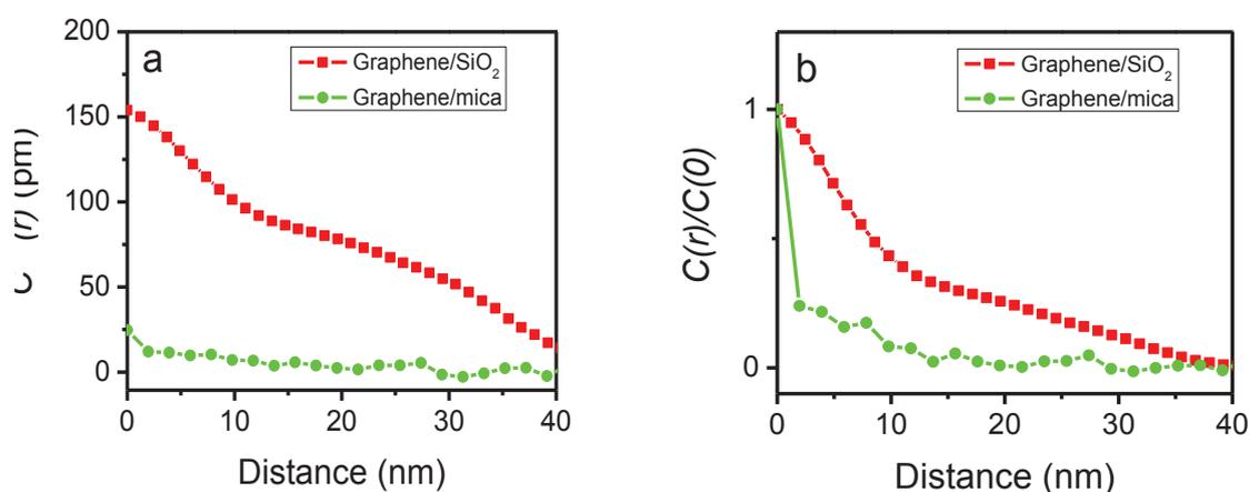
**Figure S3.** **a**, Square root of the height correlation function [ $C^{1/2}(r)$ ] for graphene/SiO<sub>2</sub> and graphene/mica. **b**, Normalized height correlation function [ $C(r)/C(0)$ ] for graphene/SiO<sub>2</sub> and graphene/mica.
