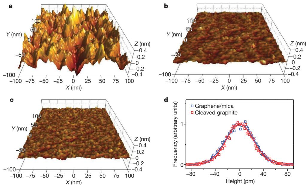
**Figure 2 | Comparison of surface roughness for graphene on SiO<sub>2</sub> and on mica, and for cleaved graphite.** **a**, **b**, Three-dimensional representations of the AFM topographic data for graphene on SiO<sub>2</sub> (**a**) and on mica (**b**) substrates. The images correspond to the regions in Fig. 1a and b designated by the blue squares. **c**, AFM image of the surface of a cleaved kish
