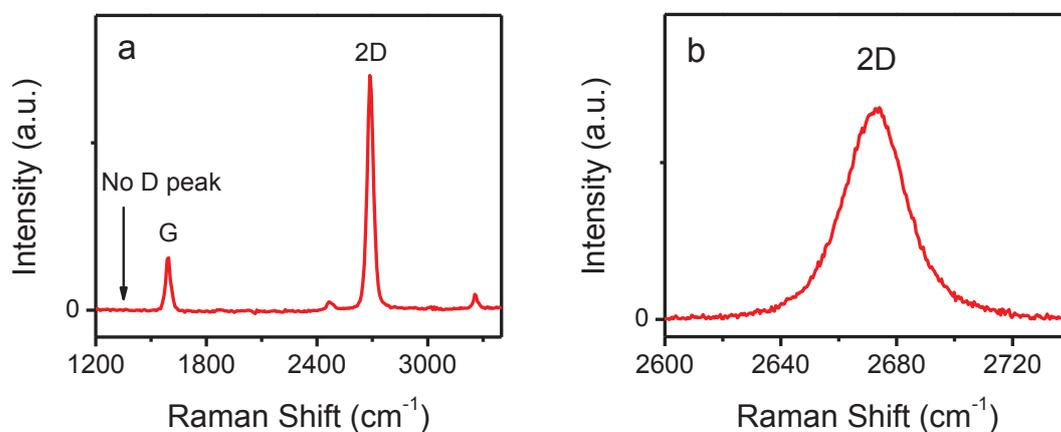
**Figure S2.** Raman spectra of the graphene monolayer in Figure S1 for an excitation wavelength of 532 nm. **a**, The Raman spectrum does not show any measurable D peak, indicating the high crystalline order of the sample. **b**, The 2D peak shows a narrow and symmetric profile, confirming that the sample is of monolayer thickness.
