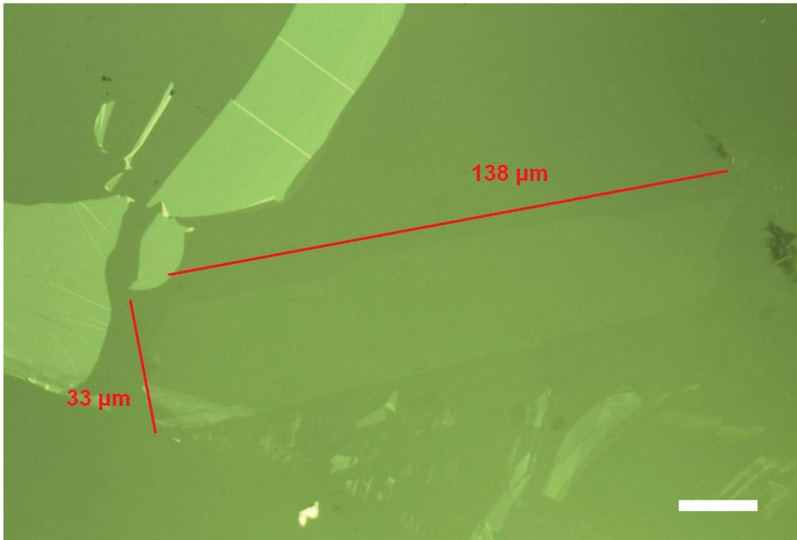
**Figure S1.** Image of a monolayer graphene sample on a mica substrate viewed by optical microscopy. The scale bar is 20  $\mu\text{m}$ .
