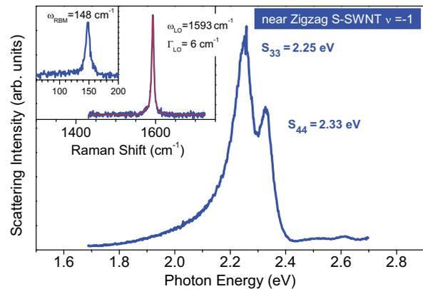
**Figure 5** (online color at: [www.pss-b.com](http://www.pss-b.com)) NTD Rayleigh and Raman spectra of a near zigzag semiconducting SWNT belonging to the  $\nu = -1$  family, assigned to (20,3) ( $d = 1.70$  nm,  $\theta = 6.9^\circ$ ) or (21,1) ( $d = 1.69$  nm,  $\theta = 2.3^\circ$ ). The Raman peaks are fit to Lorentzians. The central frequency  $\omega$  and full width at half maximum  $\Gamma$  are indicated.
