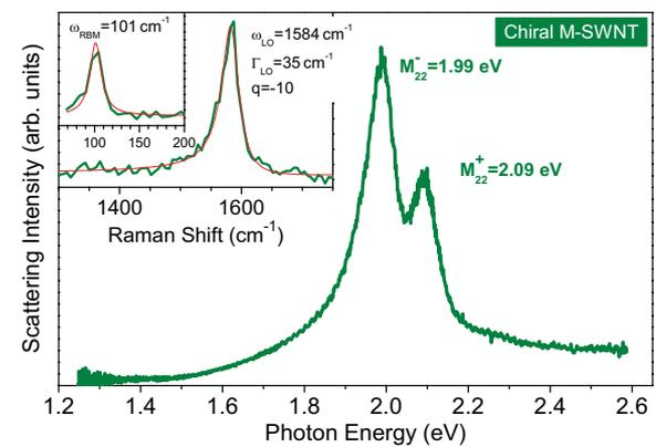
**Figure 6** (online color at: [www.pss-b.com](http://www.pss-b.com)) NTE: Rayleigh and Raman spectra of a chiral metallic SWNT assigned to (24,15) ( $d = 2.67$  nm,  $\theta = 22.4^\circ$ ). The Raman peaks are fit to Lorentzians. The central frequency  $\omega$  and full width at half maximum  $\Gamma$  are indicated.
