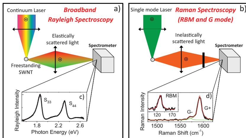
**Figure 2** (online color at: [www.pss-b.com](http://www.pss-b.com)) Micro-optical setup for (a) Rayleigh and (b) Raman scattering measurements on individual SWNTs. Typical Rayleigh (c) and Raman (d) spectra are shown for an S-SWNT (NTA) that has been assigned to (16,12) ( $d = 1.91$  nm,  $\theta = 25.3^\circ$ ). The red and green lines in (d) are Lorentzian fits of the Raman RBM and G mode features.
