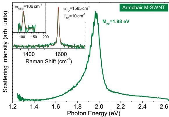
**Figure 3** (online color at: [www.pss-b.com](http://www.pss-b.com)) NTB: Rayleigh and Raman spectra of an armchair M-SWNT assigned to (19,19) ( $d = 2.58$  nm,  $\theta = 30^\circ$ ) or (20,20) ( $d = 2.71$  nm,  $\theta = 30^\circ$ ). The Raman peaks are fit to Lorentzians. The central frequency  $\omega$  and full width at half maximum  $\Gamma$  are indicated.
