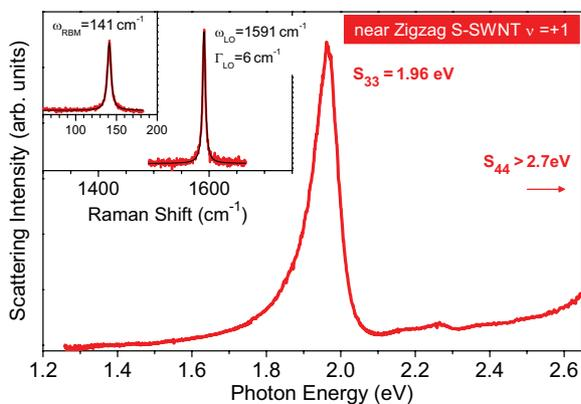
**Figure 4** (online color at: [www.pss-b.com](http://www.pss-b.com)) NTC: Rayleigh and Raman spectra of a near zigzag semiconducting SWNT belonging to the  $\nu = +1$  family, assigned to (22,0) ( $d = 1.72$  nm,  $\theta = 0^\circ$ ) or (21,2) ( $d = 1.73$  nm,  $\theta = 4.5^\circ$ ). The Raman peaks are fit to Lorentzians. The central frequency  $\omega$  and full width at half maximum  $\Gamma$  are indicated.
