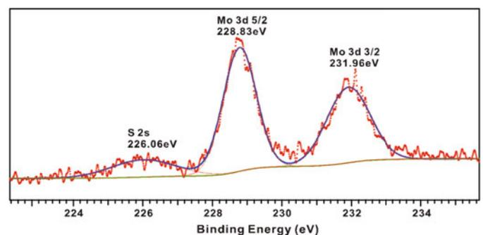
**Fig. 3.** XPS of the Mo 3d and S 2s peaks from the MoS<sub>2</sub> films on the SiO<sub>2</sub>/Si substrate.
