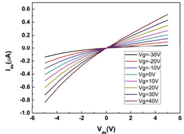
**Fig. 5.** Current-voltage (*I-V*) measurements in a 4-probe setup across a 2  $\mu$ m gap at the edge of our monolayer MoS<sub>2</sub> film as a function of gate voltage  $V_g$ . The conductivity increases for positive gate voltages, indicating *n*-type material.
