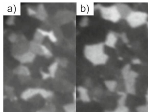
**Fig. 2.** (a, b) Spatial distribution of intensity from the MoS<sub>2</sub> (01) diffraction spot at two angular orientations  $\sim 10^\circ$  apart. The MoS<sub>2</sub> monolayer domains appear with different brightness depending on their angular orientation. Image size:  $18 \times 28 \mu\text{m}^2$ .
