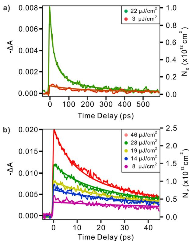
**Figure 2.** (a) Transient reflectivity of monolayer MoS<sub>2</sub> at room temperature measured at two pump fluences of 22 and 3 μJ/cm<sup>2</sup> with a time scale of 600 ps. (b) Exciton dynamics at different pump fluences with a time scale of 45 ps. The right axis corresponds to photogenerated excitons. The solid lines represent a global fit to the exciton–exciton annihilation model as seen in eq 3, by convoluting with experimental instrumental response function.
