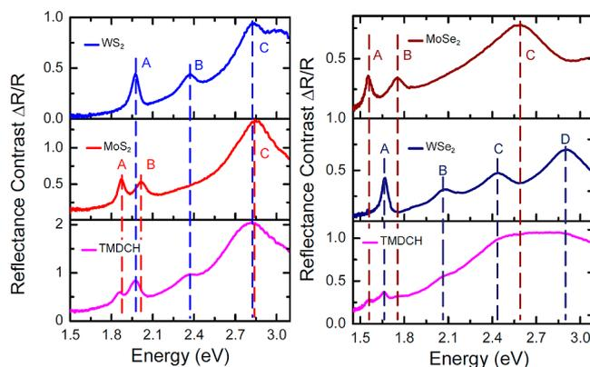
**Figure 1.** Reflectance contrast measurements for TMDCHs and their constituents, all exfoliated or transferred on fused quartz: (Left) WS<sub>2</sub> and MoS<sub>2</sub>, (Right) WSe<sub>2</sub> and MoSe<sub>2</sub>.
