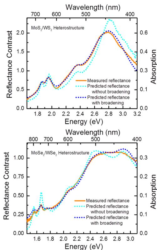
**Figure 2.** Reflectance contrast spectra of TMDCH as simulated from the dielectric functions of the respective monolayer constituents with (blue dotted line) and without (cyan dotted line) additional peak broadening are compared with the measured data (orange solid line) for (top) MoS<sub>2</sub>/WS<sub>2</sub> and (bottom) MoSe<sub>2</sub>/WSe<sub>2</sub> TMDCH heterostructures. Absorption is calculated with the methods in ref 30.
