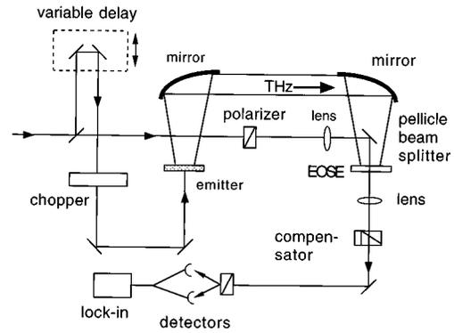
FIG. 2. Schematic drawing of the experimental setup used to detect freely propagating THz radiation.  $\langle 110 \rangle$  ZnTe was used to generate THz radiation by optical rectification and detect THz radiation by electro-optic sampling.
