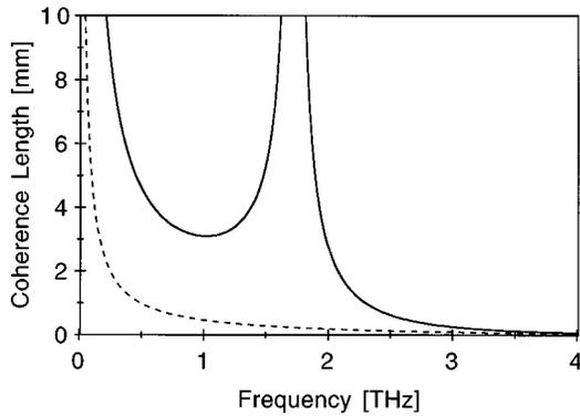
FIG. 1. Coherence length vs THz frequency for ZnTe using optical excitation at 800 nm. The dotted line, calculated using Eq. (2), neglects the dispersion at optical frequencies. The solid line, calculated using Eq. (6), includes the effects of dispersion at optical frequencies.
