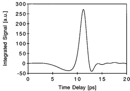
FIG. 5. Temporal integration of the wave form shown in Fig. 4.
