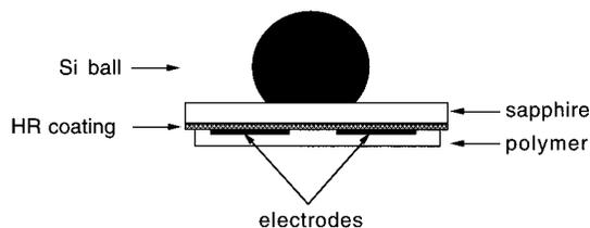
FIG. 1. Schematic drawing of the electro-optic sampling element.
