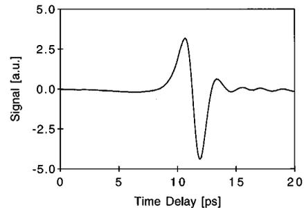
FIG. 4. Temporal wave form obtained with a 100  $\mu\text{m}$  Hertzian dipole detector that preserves the bipolar nature of the incident THz field. The experimental conditions were identical to those used for the electro-optic sampling measurement.
