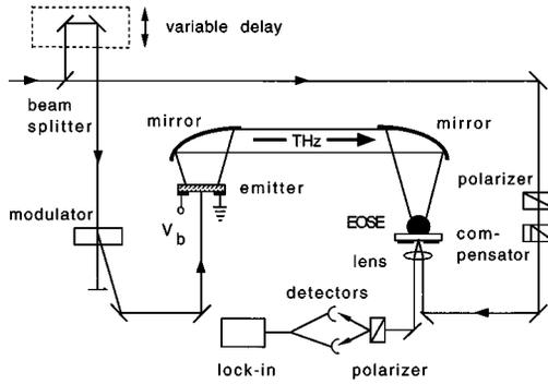
FIG. 2. Schematic drawing of the experimental setup used to detect freely propagating THz radiation.
