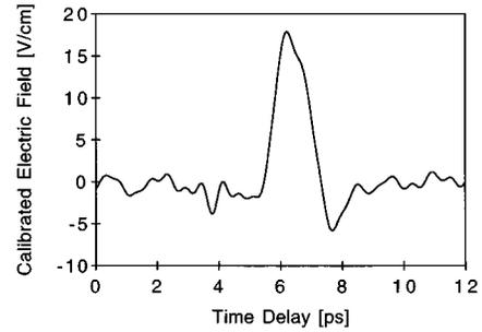
FIG. 3. Temporal wave form detected by electro-optic sampling.
