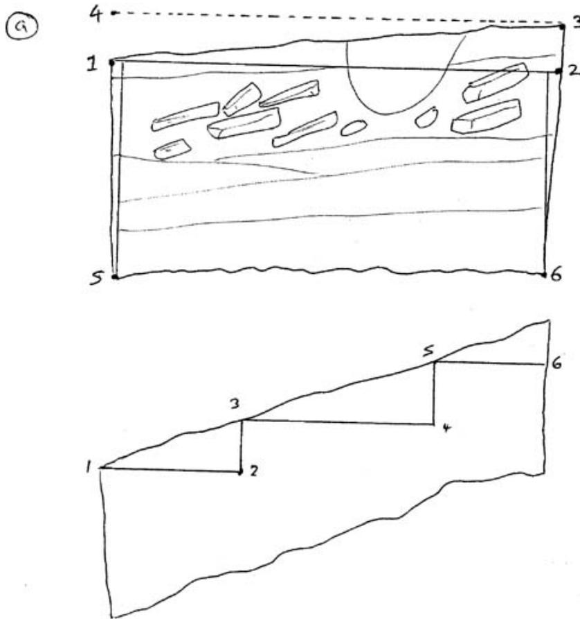
Next, measure along your string from point 1, and mark it at 1-meter or 50-centimeter intervals. Drive pegs into the wall of the trench, with the distances marked on them. Don't attach a tape measure or line-level to your string, because the weight of these will pull the string down so that it's no longer level.
