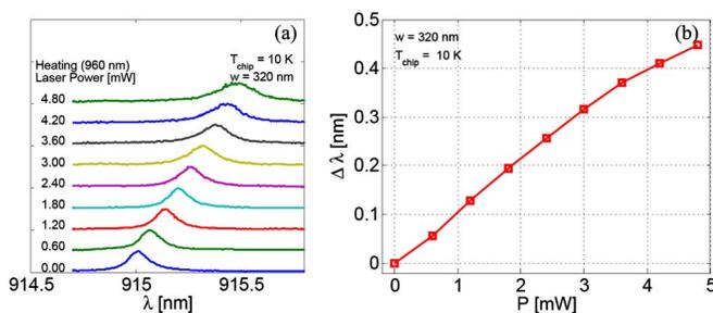
FIG. 3. (Color online) (a) Detuning of the PC cavity resonance with increasing temperature due to local heating. (b) Dependence of the PC cavity resonance wavelength on the local heating power.
