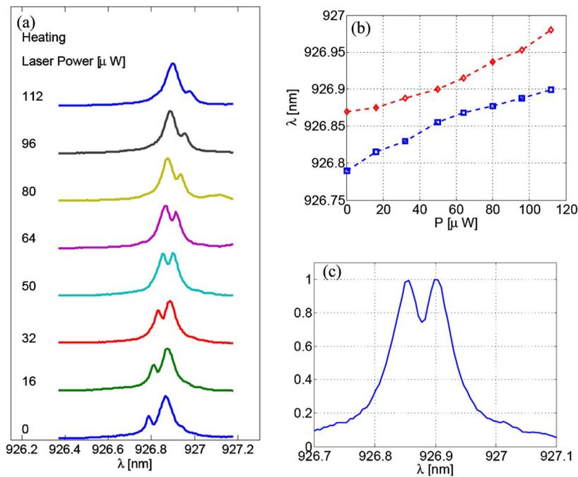
FIG. 4. (Color online) (a) Spectra showing the tuning of a single QD into resonance with the cavity mode using the local heating technique. (b) Anticrossing between the polariton lines of the strongly coupled PC cavity-QD system. (c) Spectrum showing the 0.05 nm splitting of the polaritons. Note that the data in this figure were taken on a different chip than the data in Figs. 1–3.
