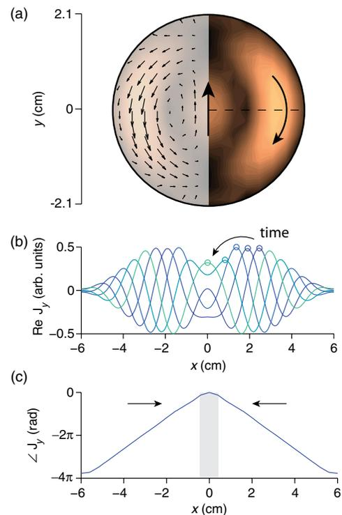
FIG. 3 (color online). (a) A reduced view of the optimal current density composed of three current paths. (b) Change in current density with time along an axial cut (dotted line) over a half-period. (c) Spatial phase variation shows that the center is stationary (constant region, shaded) while currents away from the center propagate inwards (linear region, nonshaded).
