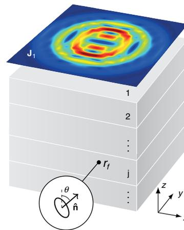
FIG. 1 (color online). The general configuration for wireless power transfer consists of a source surface current density  $\mathbf{J}_1$  and a receive coil positioned in tissue with magnetic dipole moment  $\hat{\mathbf{n}}$  at an angle  $\theta$ . The tissue geometry is modeled by multilayers. By convention, the dipole moment aligns with the  $z$  axis when  $\theta = 0^\circ$ , and the  $x$  axis when  $\theta = 90^\circ$ .
