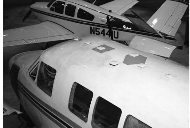
Figure 15. Antenna Installation on the Queen Air Test Airplane
