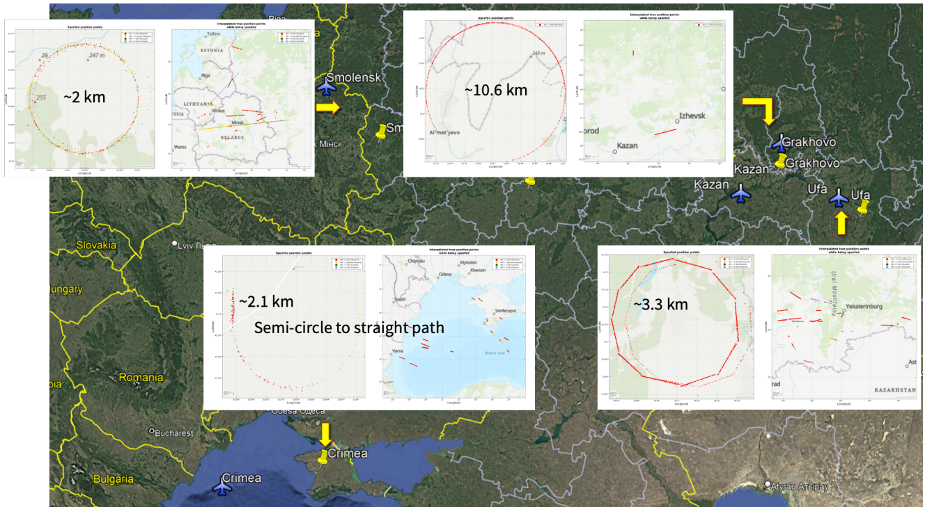
FIGURE 5. Other spoofing seen in Russia, March 2025. 4 distinct events are shown in the inserts with the rough diameter of the largest spoof “circle” in each event (left plot) and estimated positions during spoof (right plot)
