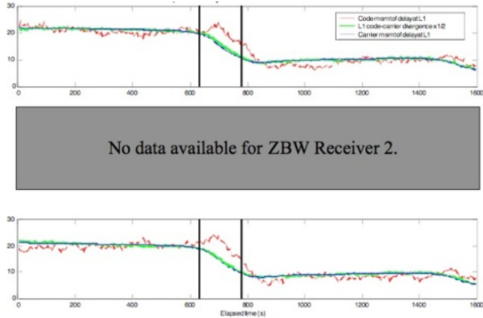
Figure 5.7: Slant ionospheric delay in meters to SVN 24 from each receiver at Boston WAAS station. Data for Receiver 2 not available.
