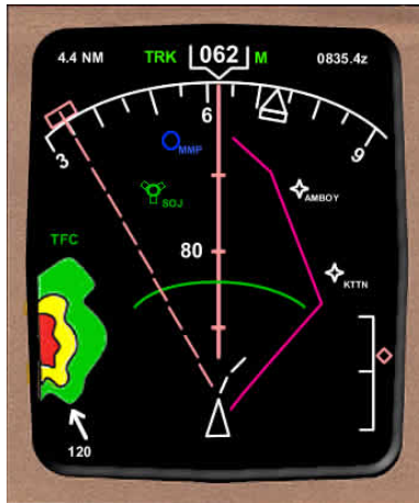
Figure 12.1 Boeing's green arc indicates the horizontal position at which altitude capture occurs using a simple linear extrapolation algorithm.
