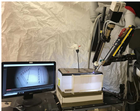
Fig. 2. The full experimental setup of the standard laparoscopic surgery training study: a modified PSM of a first-generation da Vinci is on the right along with the PSM that holds the da Vinci camera. The white handle in the middle is the traditional laparoscopic tool. This tool, along with the camera and the PSMs are all inserted into a laparoscopic box trainer in the middle. A monitor showing what is inside the box is on the left.
