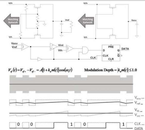
Figure 17.6.4: Demodulator schematic along with the description of the asynchronous pulse-width ASK modulation. The equation describes amplitude modulation, with modulation depth as defined.
