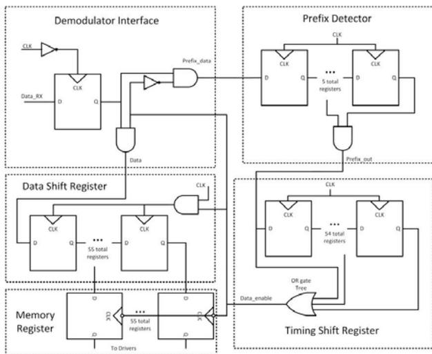
Figure 17.6.5: Digital controller schematic depicting the operation of the data receive circuitry.
