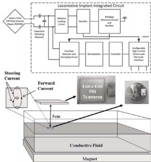
Figure 17.6.1: System-level block diagram of the implantable device, and magnetohydrodynamic propulsion experimental setup.
