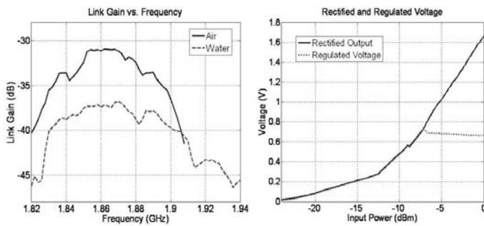
Figure 17.6.3: Measured link gain at the input of the antenna when in air and on top of water, and the rectified and regulated voltage as a function of input power.
