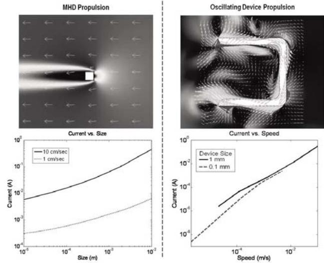
Figure 17.6.2: Performance summary of the electromagnetic propulsion mechanisms determined with numerical fluid simulations.
