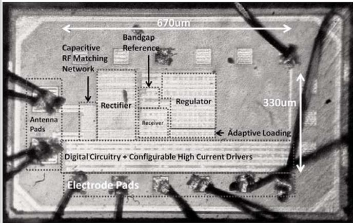
Figure 17.6.7: Chip die photo, total area including pads is 0.6mm<sup>2</sup>.
